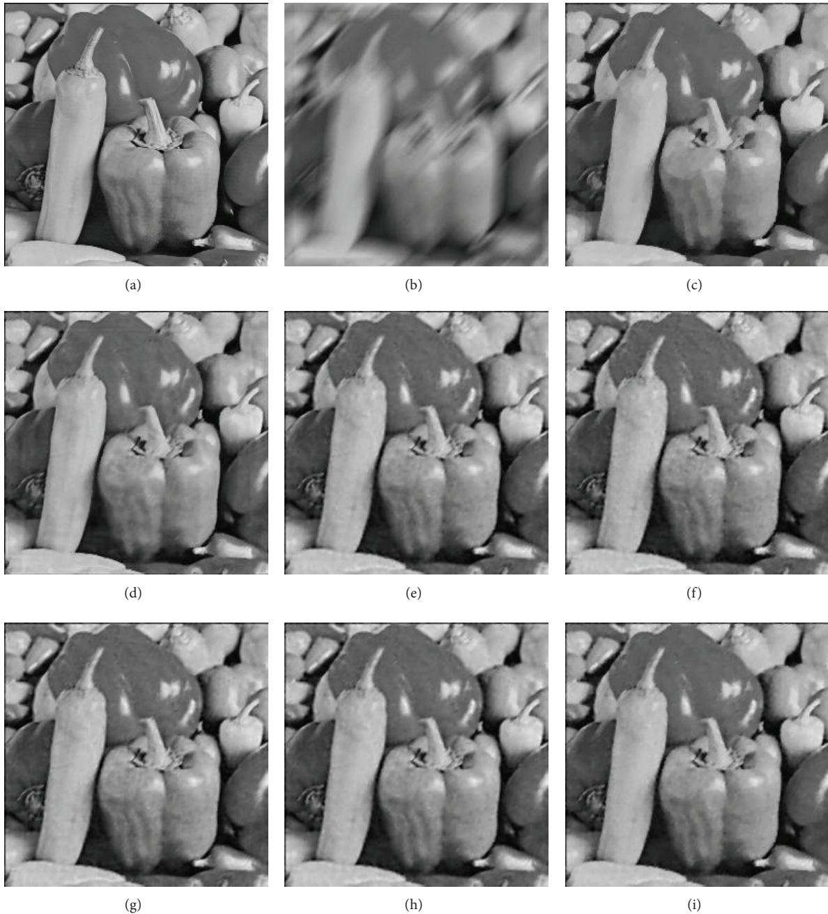
FIGURE 5: Results of different methods on the Peppers image degraded by motion blurring and noise corresponding to a BSNR level of 30 dB: (a) original image, (b) degraded image (PSNR = 18.98 dB), (c) TV solution (PSNR = 27.19 dB), (d) nonlocal TV solution (PSNR = 27.64 dB), (e) Hessian Frobenius-norm solution (PSNR = 28.15 dB), (f) Hessian Spectral-norm solution (PSNR = 27.97 dB), (g) Hessian Nuclear-norm solution (PSNR = 28.16 dB), (h) ISDTV solution (PSNR = 28.11 dB), and (i) MHOTV solution (PSNR = 28.66 dB).
