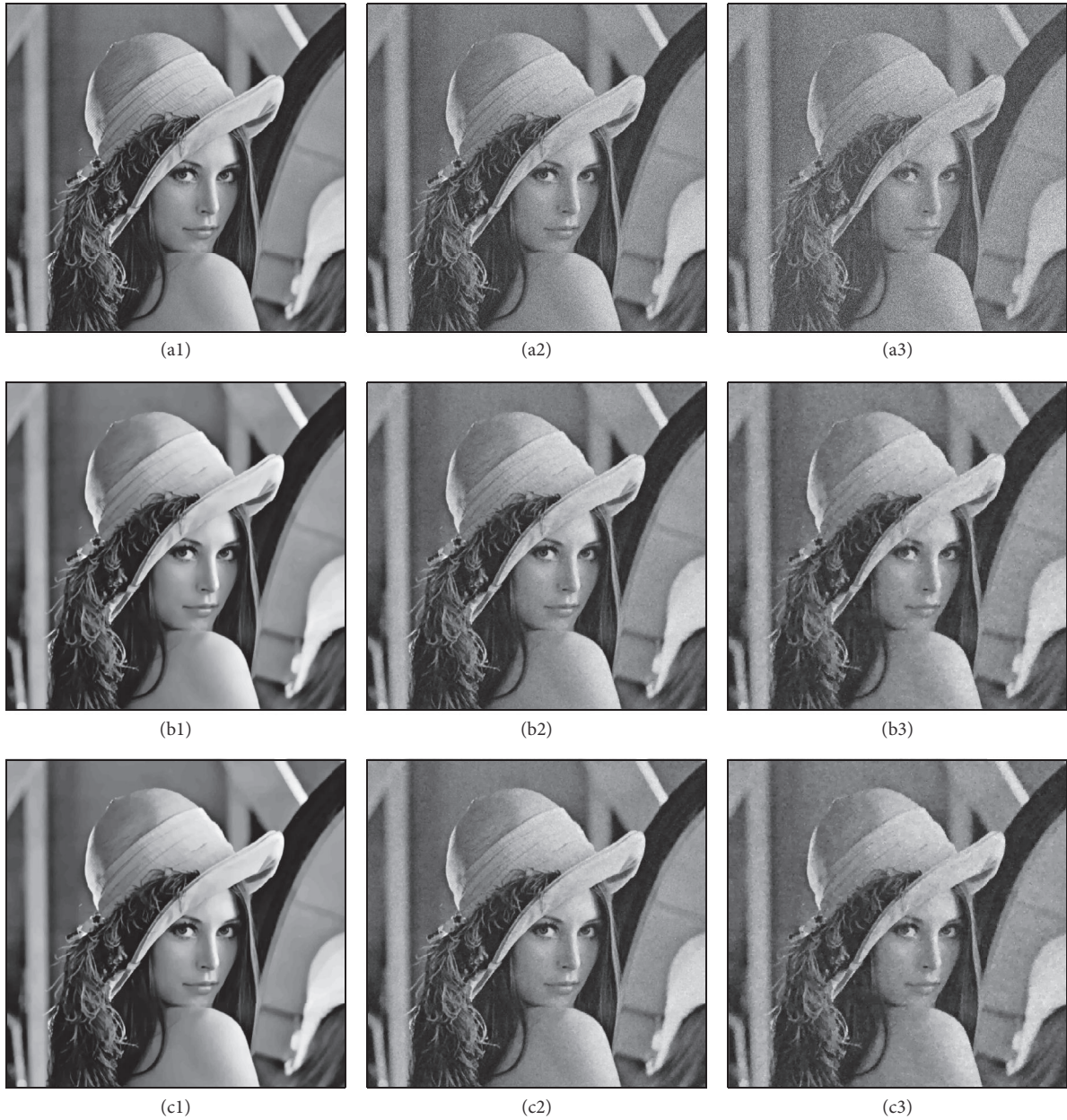
FIGURE 6: (a1)–(a3) are the noisy image of “Lena” with noise levels 0.01, 0.05, and 0.1, respectively; (b1)–(b3) are the denoised image by Algorithm 1; (c1)–(c3) are the denoised image by our proposed Algorithm 4.
