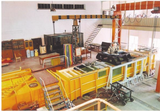
FIGURE 5: Circulating water flume for hydrodynamic tests.
