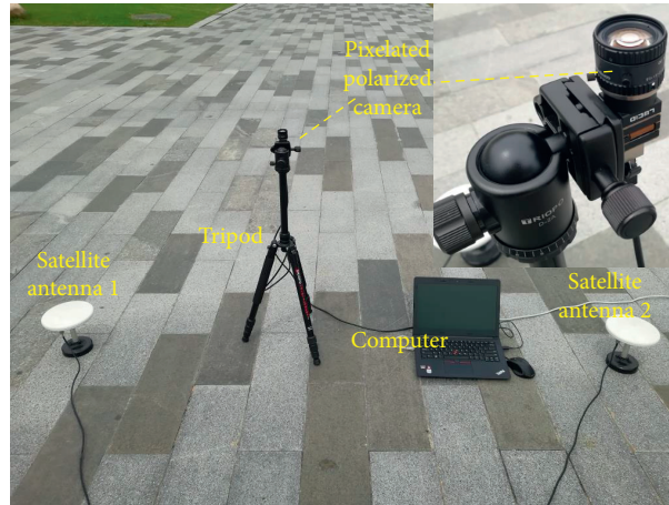
FIGURE 12: Polarized skylight navigation platform.
