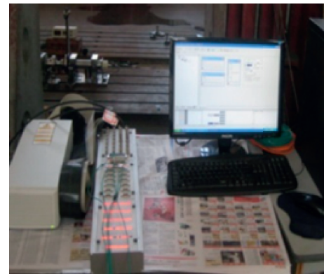
FIGURE 11: dSPACE signal collection system.
