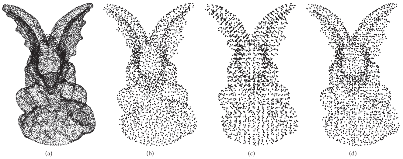
FIGURE 9: Gargo50 K simplification results. (a) Gargo50 K. (b) Grid sampling. (c) Poisson-disk sampling. (d) MFCM.
