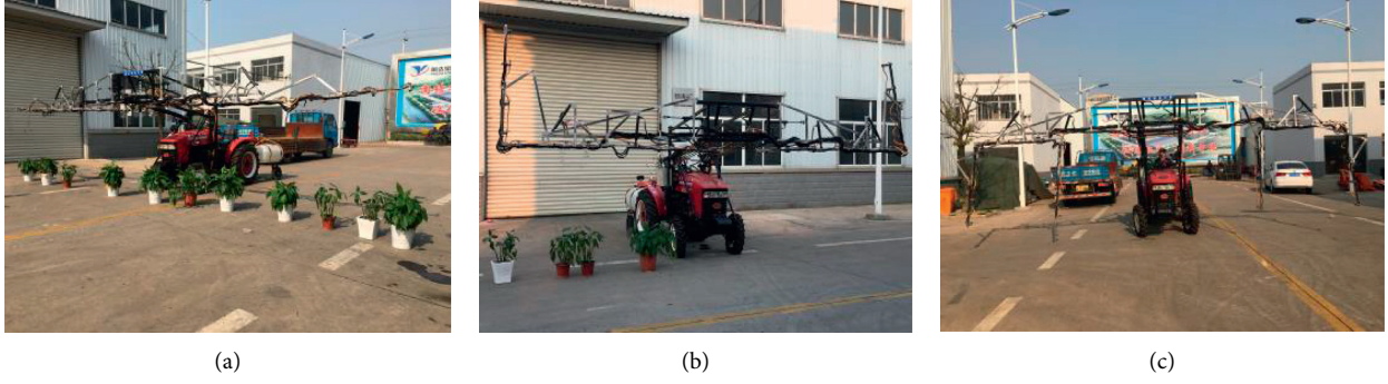
FIGURE 2: Reconfiguration images of the multifunctional shiftable boom intelligent sprayer. (a) The shape of “—.” (b) The shape of “U.” (c) The shape of “fl.”
