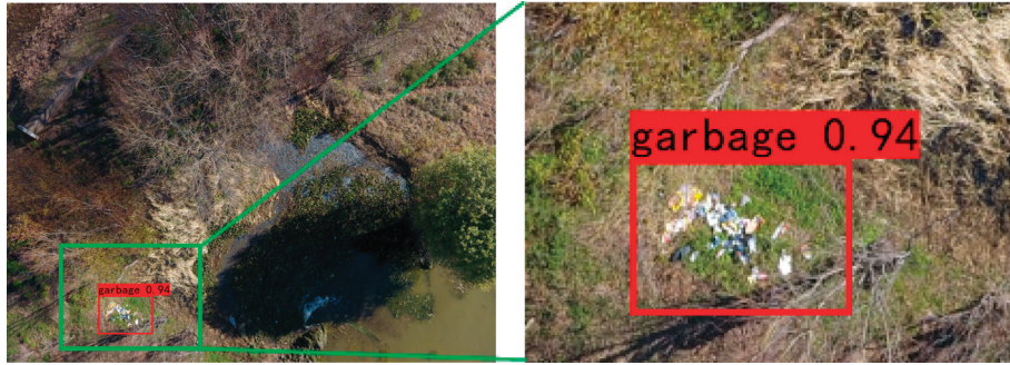
FIGURE 1: A garbage scattered area sample is detected in the remote sensing image. This sample is collected in Dali Cangshan Erhai Nature Reserve. The area of the green bounding box is enlarged and displayed.
