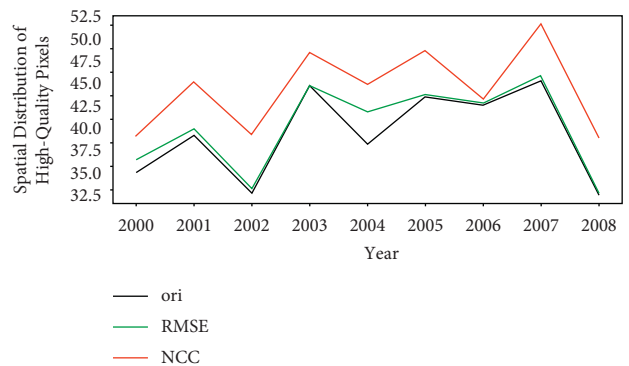
FIGURE 6: Proportion of “good quality” pixels at altitudes 500 m–1500 m (RMSE and NCC).
