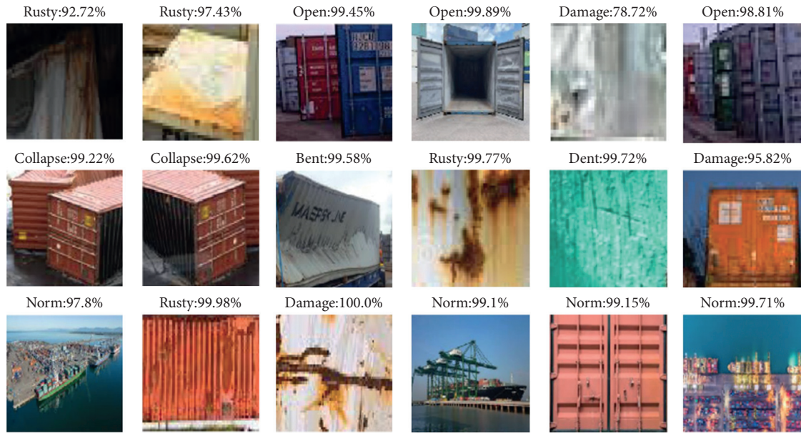
FIGURE 7: Test results of the detection model. It shows the result of the damage test of the container extracted at random.
