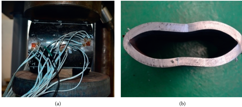
FIGURE 5: Installation diagram of sample 1-1 before the test (a) and shape of sample 1-1 after the test (b).
