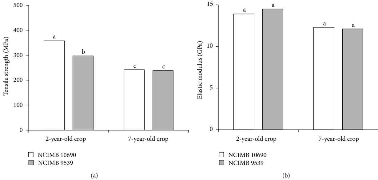
FIGURE 2: Influence of crop age and microbial strain on tensile strength (a) and elastic modulus (b). Mean values followed by the same letters are not significantly different for  $P \leq 0.05$  following a two-way ANOVA test with crop age and microbial strain as variability factors.
