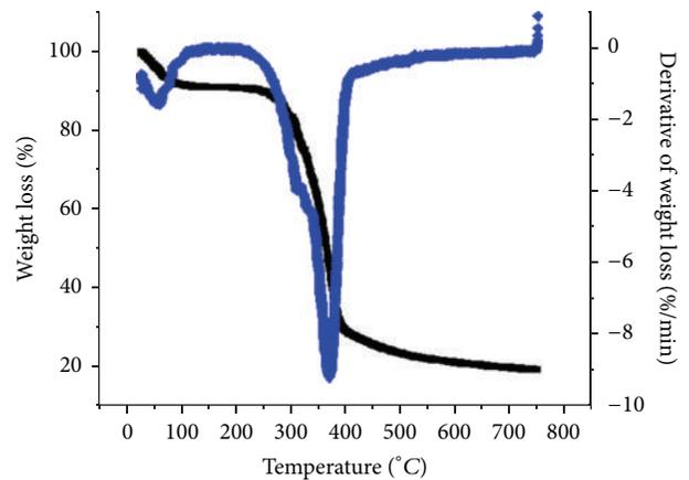
FIGURE 5: Thermogravimetric behavior of the *H. bihai* fiber. The same overall behavior was also observed for *E. elatior* and *C. comosus* fibers.
