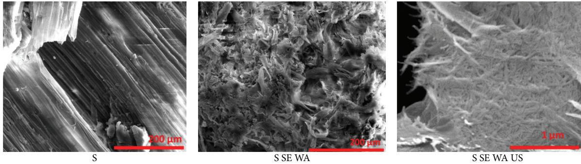
FIGURE 3: Untreated, steam-exploded, and ultrasonic-treated hemp.
