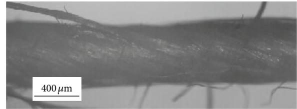
FIGURE 6: Water-treated yarn with tension.
