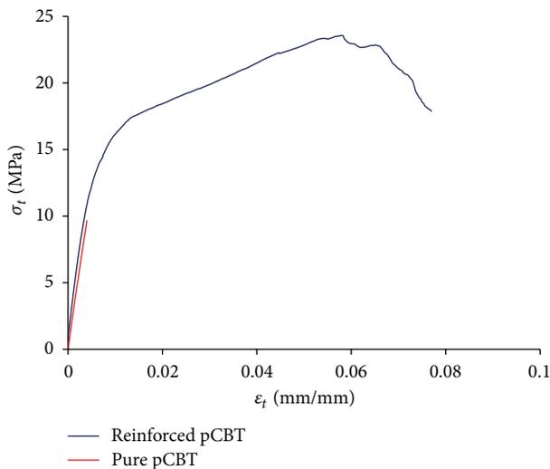
FIGURE 5: Typical tensile stress—strain plots for pure and reinforced pCBT.
