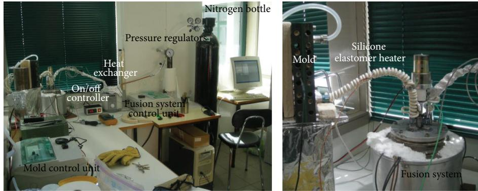
FIGURE 3: The developed RTM set-up.
