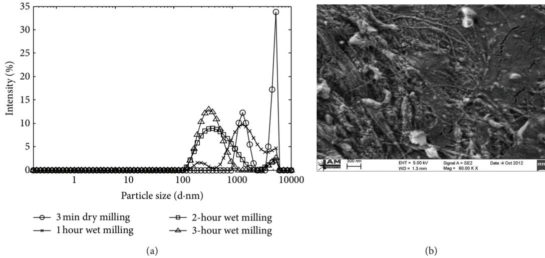
FIGURE 3: (a) Effect of extended wet milling time on pulverization. (b) FESEM image of particle size after 3-hour wet milling.
