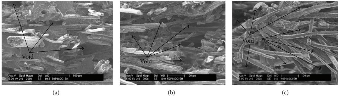
FIGURE 6: SEM micrographs of impact fracture surface of 40% (a), 50% (b), and 60% (c) flax fibre reinforced composites.
