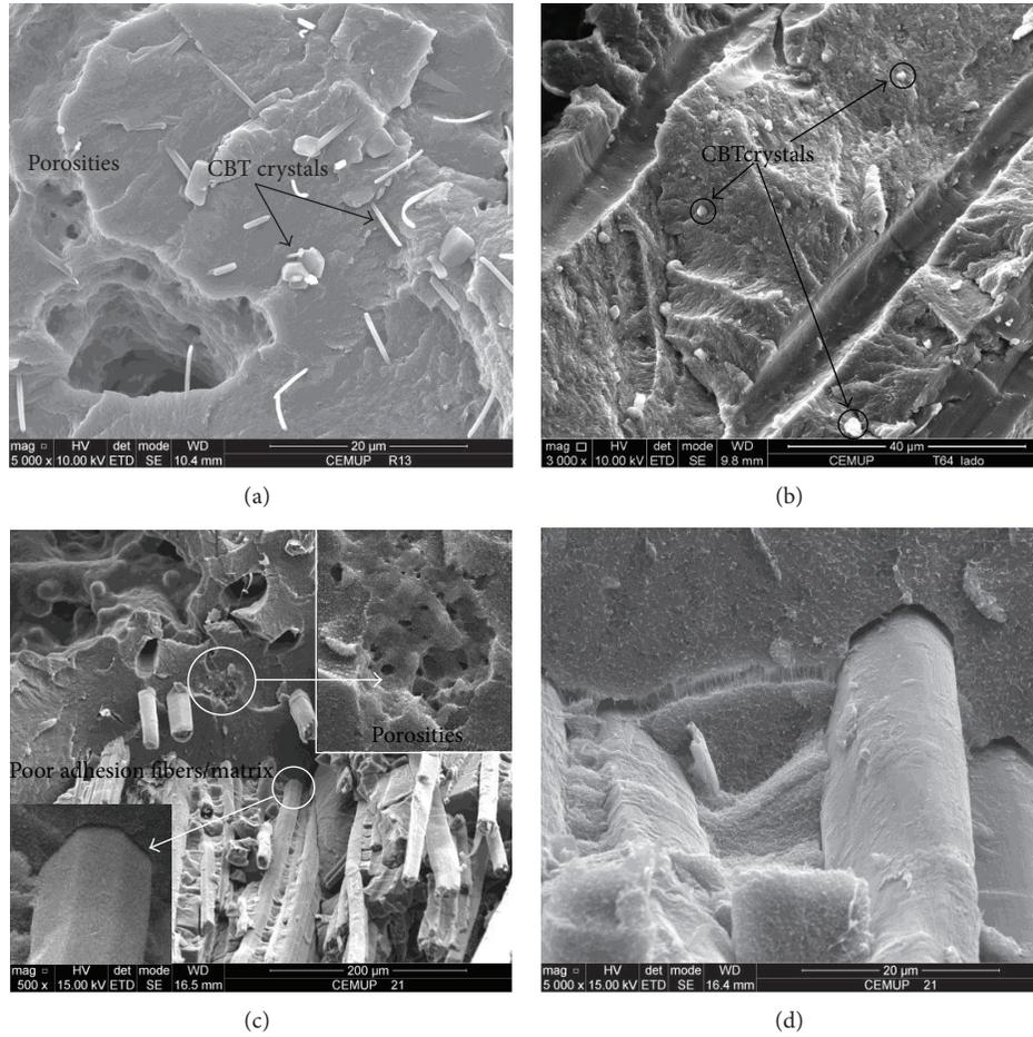
FIGURE 6: SEM micrographs of neat pCBT (a) and flax reinforced pCBT ((b), (c), and (d)).
