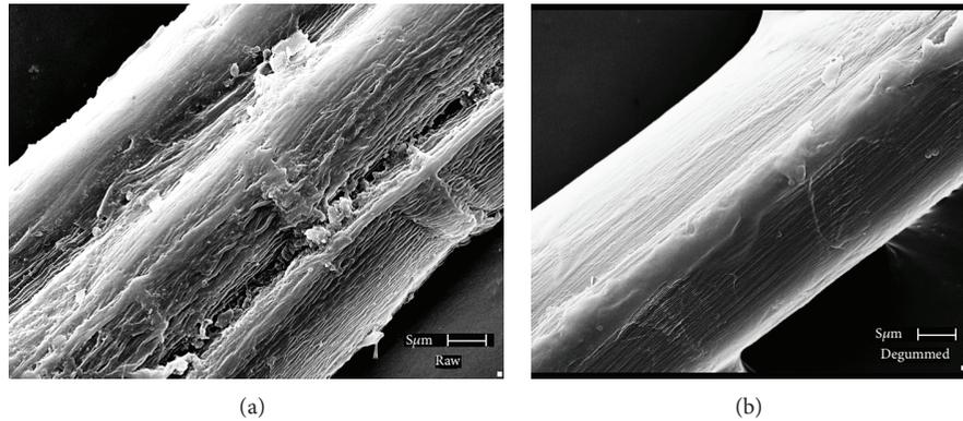
FIGURE 1: SEM of raw and degummed ramie.
