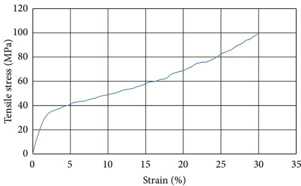
FIGURE 3: Representative stress-strain curve showing the tensile behavior of coir fibres.
