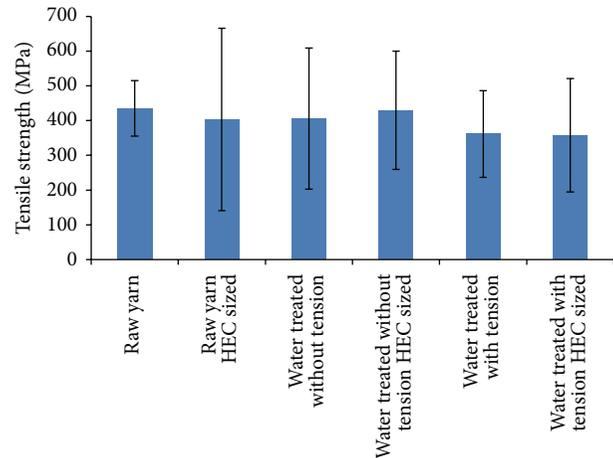
FIGURE 1: Tensile strength of single jute fibre (error bars indicate standard deviation).
