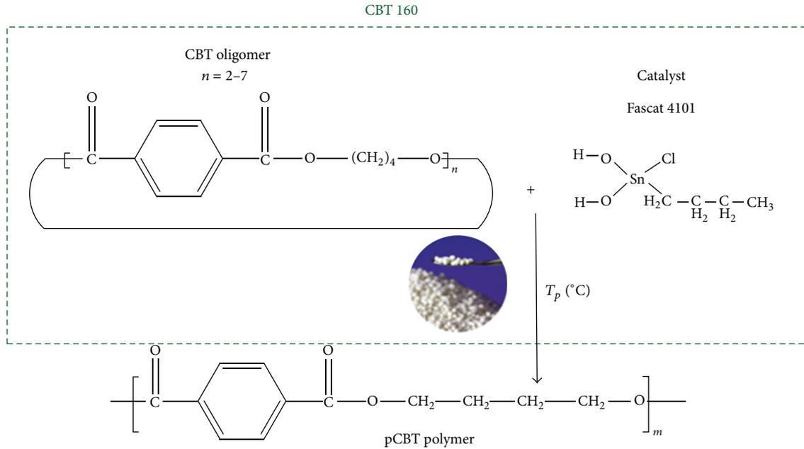
FIGURE 1: CBT 160 resin and its polymerization to pCBT (polymerized CBT).
