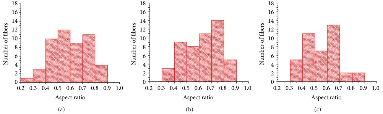
FIGURE 6: Aspect ratio histograms from (a) *E. elatior*, (b) *C. comosus*, and (c) *H. bihai* fibers.
