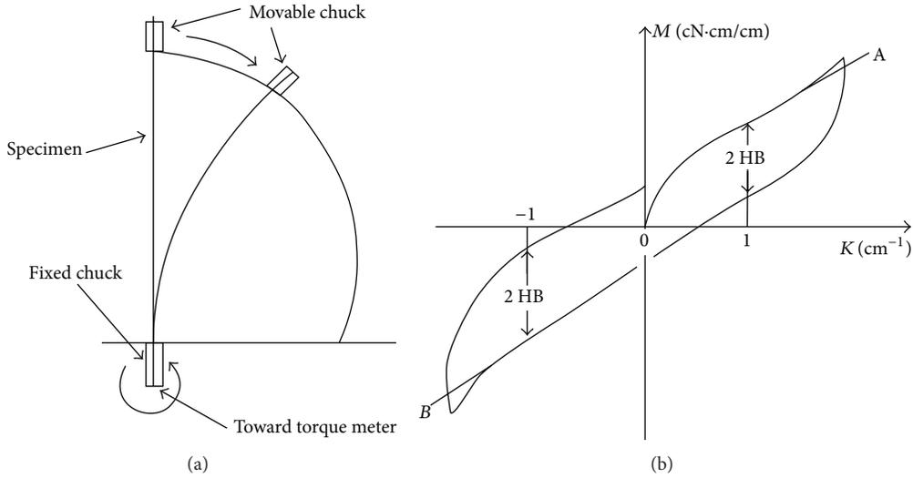
FIGURE 1: KES-FB2 diagram (a) and bending diagram (b) [11].
