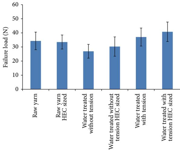
FIGURE 3: Failure load of single jute yarn (error bars indicate standard deviation).
