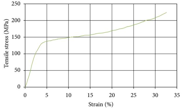
FIGURE 5: Representative curves for tensile behaviour of some of the tested horsetail hair fibres.
