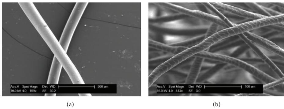
FIGURE 11: SEM images showing the smooth surface of cattle hair (a) versus keratinous structure of wool (b).
