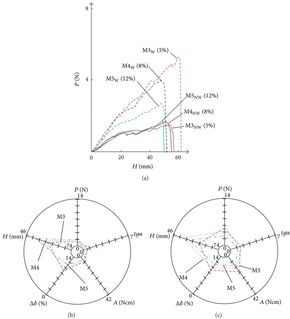
FIGURE 3: Typical pulling curves of viscose knitted materials with different elastane content (a); the diagrams of complex hand rates  $Q_{NW}$  calculation for nonwashed specimens (b); the calculation of complex hand rates  $Q_W$  after sample washing (c).
