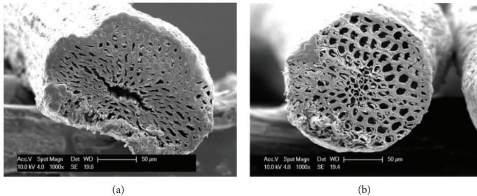
FIGURE 9: SEM images of the cross-sections of coir fibres.
