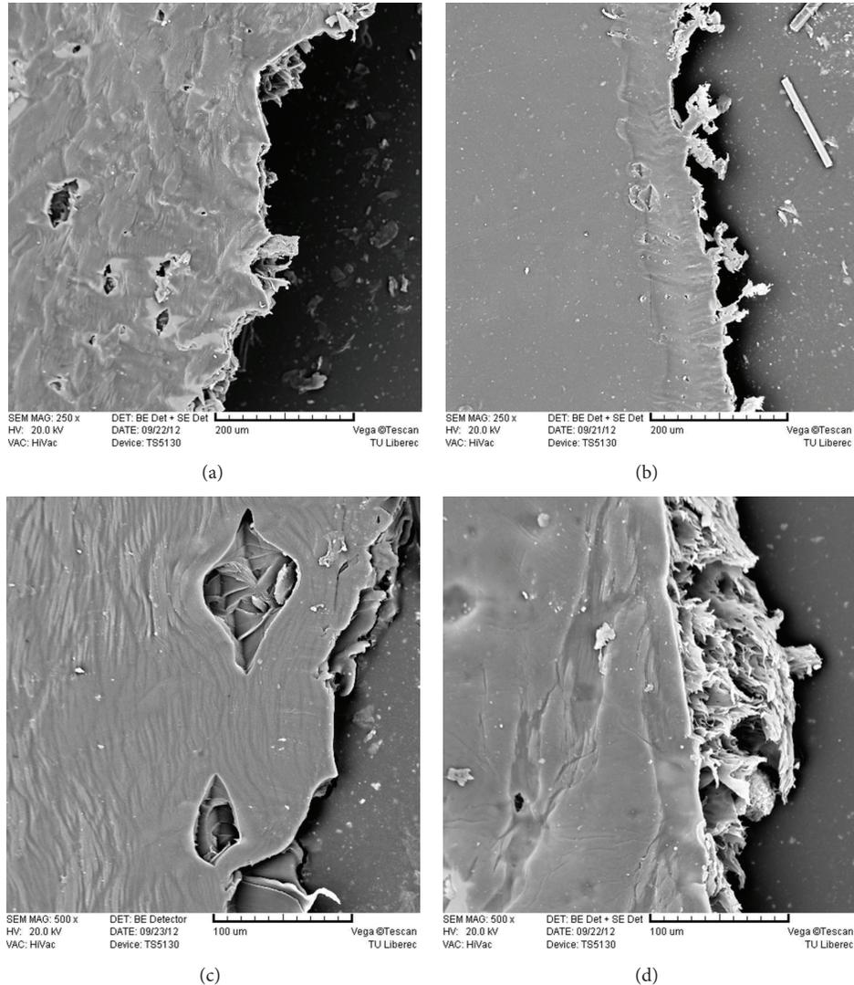
FIGURE 6: (a) Neat PLA film. (b) 1% JNF/PLA film. (c) 5% JNF/PLA film. (d) 10% JNF/PLA film.
