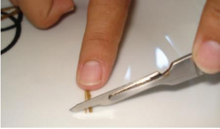
FIGURE 1: Procedure used to obtain sharp cross-section. After soaking the fibers in water, the use of a doctor blade enables a cut without deformation artifacts due to the cutting procedure.
