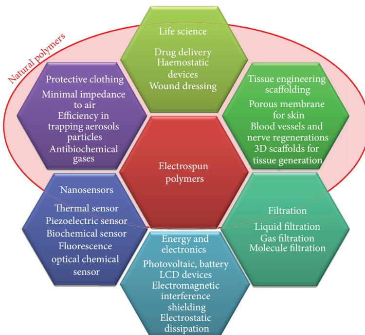
FIGURE 3: A selection of potential applications for electrospun polymer systems, highlighting the current areas of most interest for natural polymers.
