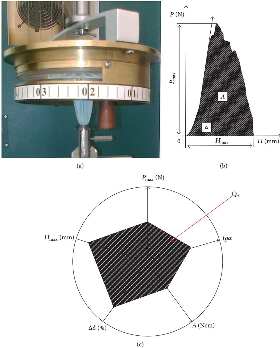
FIGURE 1: KTU-Griff-Tester device (a); typical extraction curve  $H$ - $P$  (b); the optimisation diagram (c).
