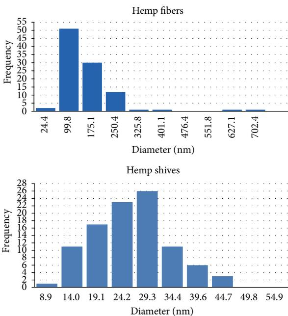
FIGURE 4: Size distribution of steam-exploded and ultrasonic-treated hemp fibers and shives diameter.
