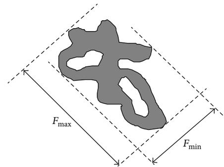
FIGURE 3: Definition of the size parameters of an object.
