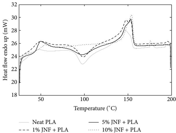
FIGURE 4: DSC of neat PLA and nanocomposite films.
