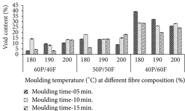
FIGURE 5: Effect of process variables on the void content of the biocomposites.
