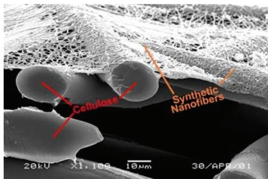
FIGURE 8: AMSOIL Ea air filters used for automotive industry [93].
