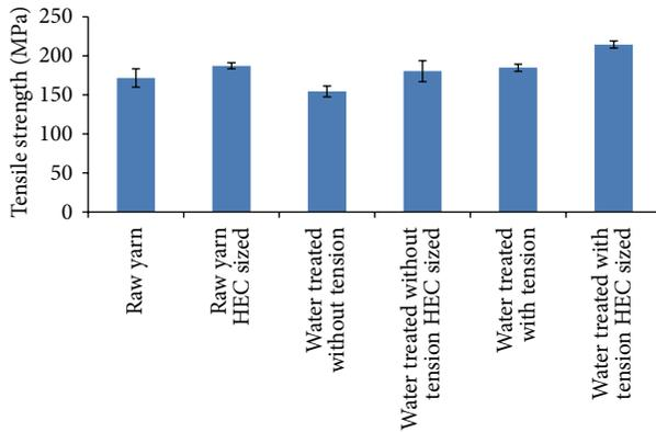
FIGURE 10: Tensile strength of composites (error bars indicate standard deviation).
