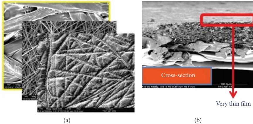
FIGURE 7: A three-tier architecture of TFNC membrane (a) and its cross-sectional view (b) [84].
