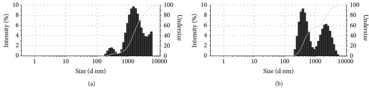
FIGURE 1: (a) Particle size distribution of one hour dry milling. (b) Particle size distribution of one hour wet milling.
