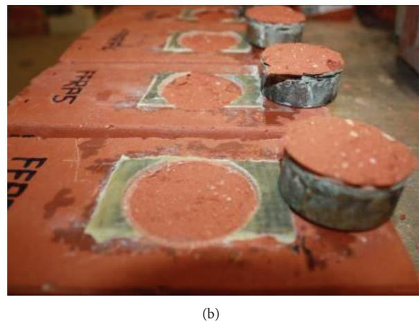
FIGURE 6: (a) Schematic failure modes for PT and (b) specimens tested.
