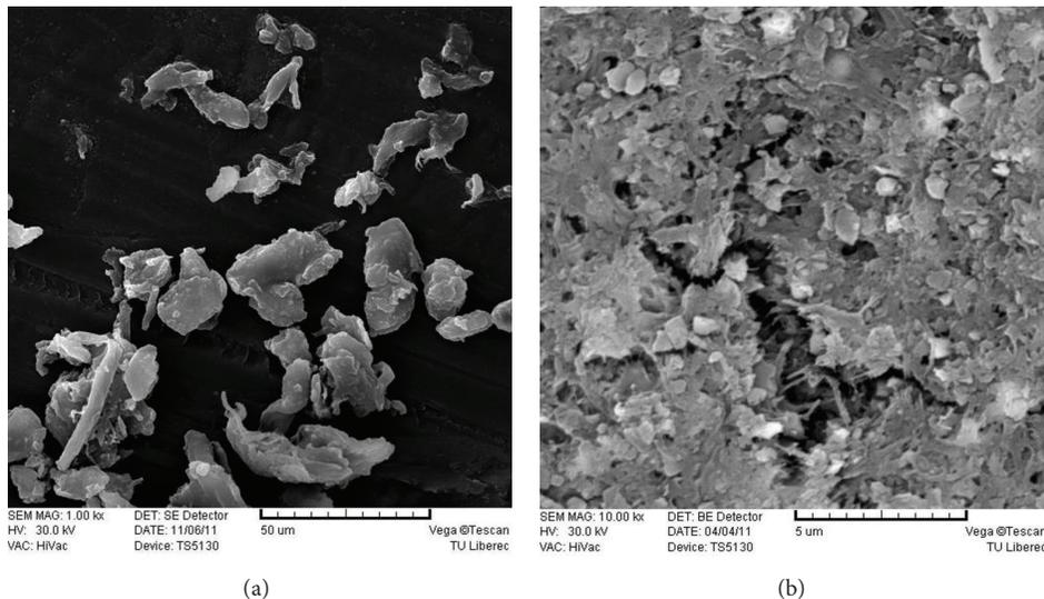
FIGURE 2: (a) SEM image of one hour dry milling. (b) SEM image of one hour wet milling.
