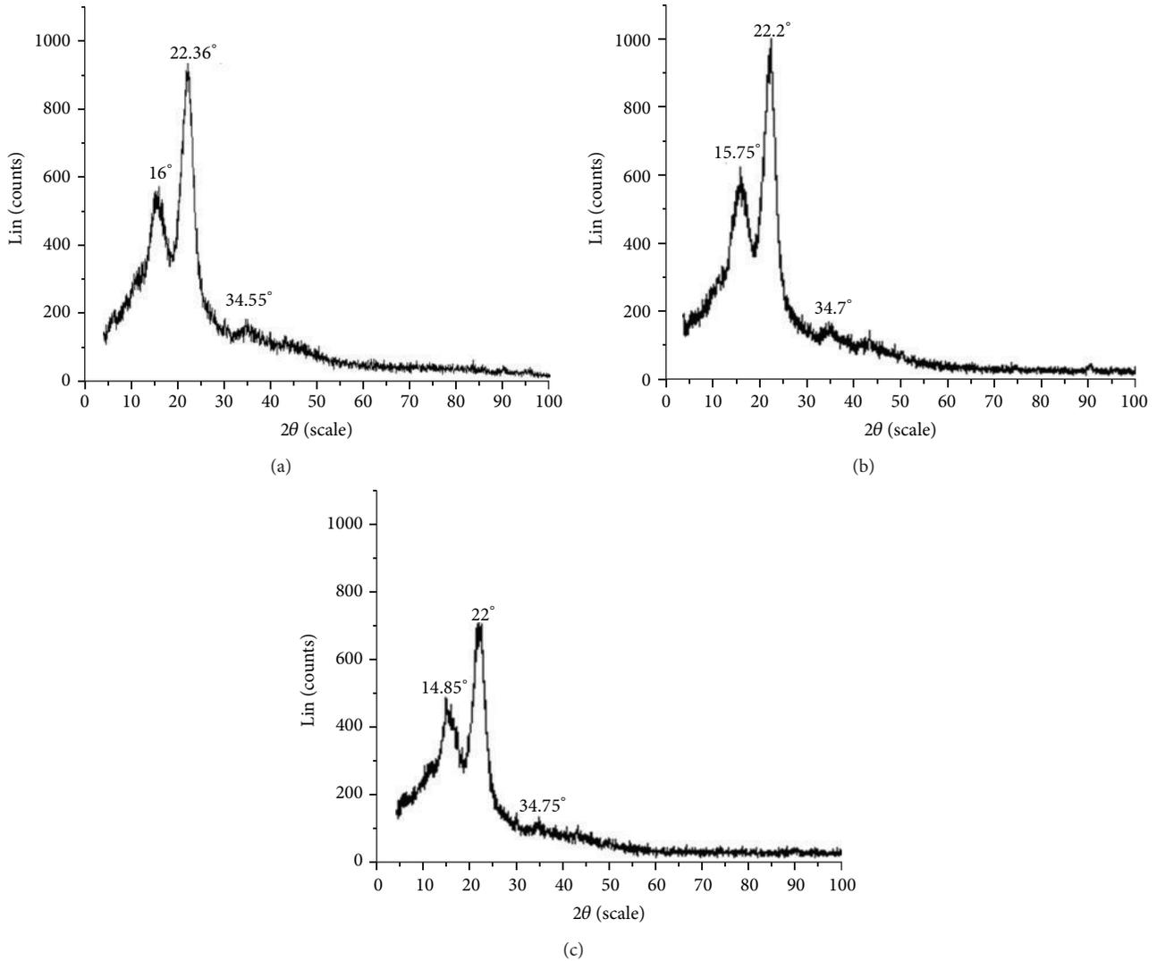
FIGURE 4: X-rays diffractogram of the fibers: (a) *E. elatior*; (b) *C. comosus*; and (c) *H. bihai*.
