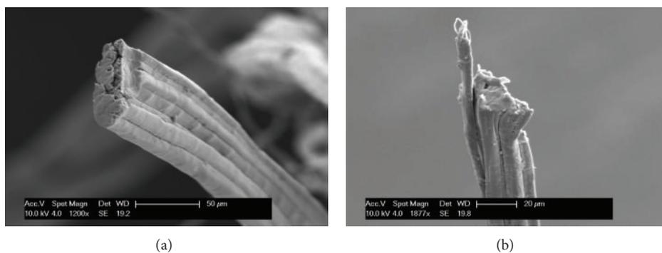
FIGURE 13: Jute fibres shown to consist of several elementary fibres waxed together.
