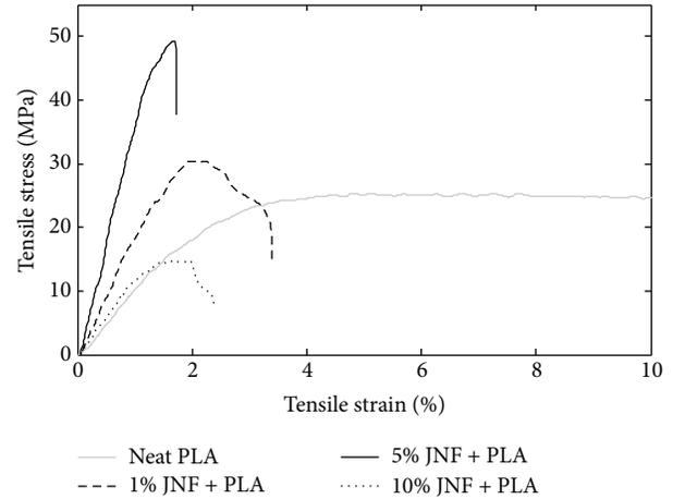
FIGURE 5: Stress-strain curve of neat PLA and nanocomposite films.
