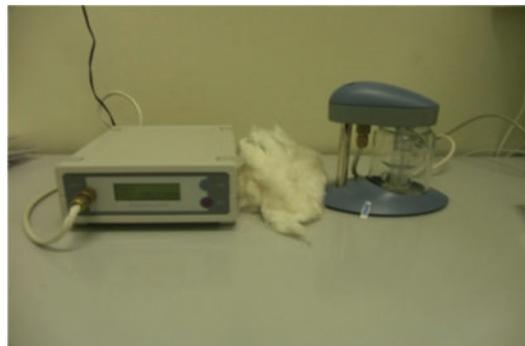
FIGURE 1: Biosensor toxicity analyzer with microflow unit.
