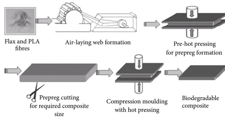
FIGURE 1: Schematic diagram of composite manufacturing steps.
