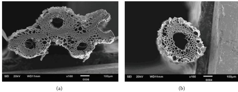
FIGURE 7: Examples of the large fibers' cross-section variability found for *C. comosus*.
