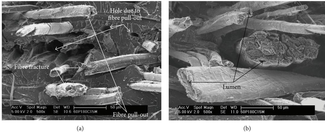
FIGURE 4: SEM micrograph of the impact fracture surface of the biocomposite. (a) The fibre fracture and fibre pull-out. (b) The lumen in the flax fibre.
