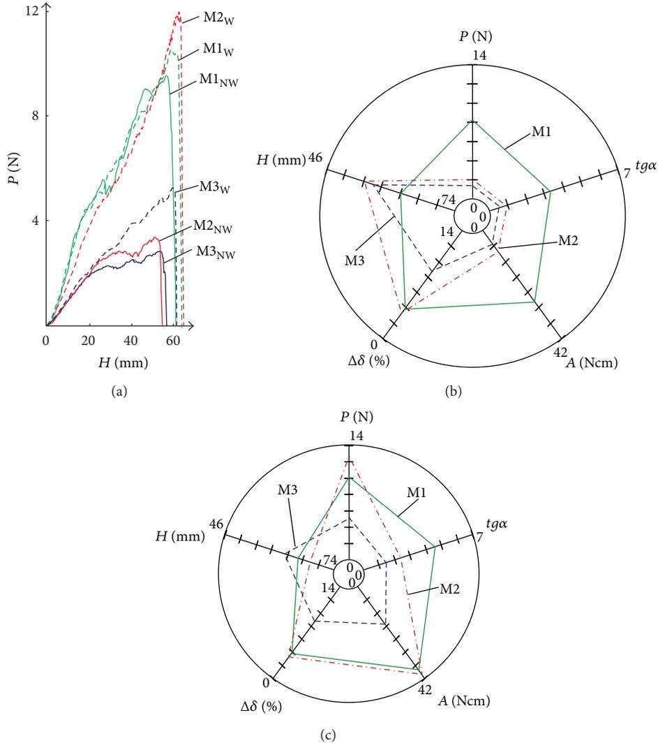
FIGURE 2: Typical pulling curves of knitted materials with different fibre content (a); the diagram of complex hand rates  $Q_{NW}$  calculation for nonwashed specimen (b); the calculation of complex hand rates  $Q_W$  after sample washing (c).
