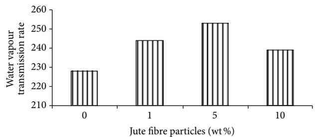
FIGURE 7: Moisture barrier of neat PLA and nanocomposite film.
