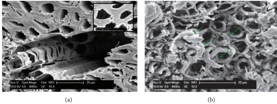
FIGURE 10: SEM images showing (a) coir microfibrils at higher magnification with the spring-like structure and the interconnecting layer and (b) fracture surface of a coir fibre that failed under tensile loading (the arrows point towards features demonstrating spirality of the microfibrils).
