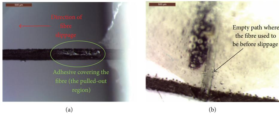
FIGURE 2: Optical microscope images of coir fibre under tensile loading slipping out of the adhesive (a), and the adhesive after the fibre has slipped out with its empty space clearly obvious (b).
