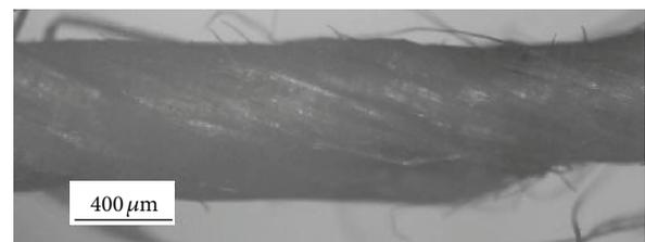
FIGURE 9: Water-treated yarn with tension.
