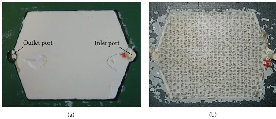
FIGURE 4: Pure pCBT (a) and flax reinforced pCBT (b) plates produced by RTM.
