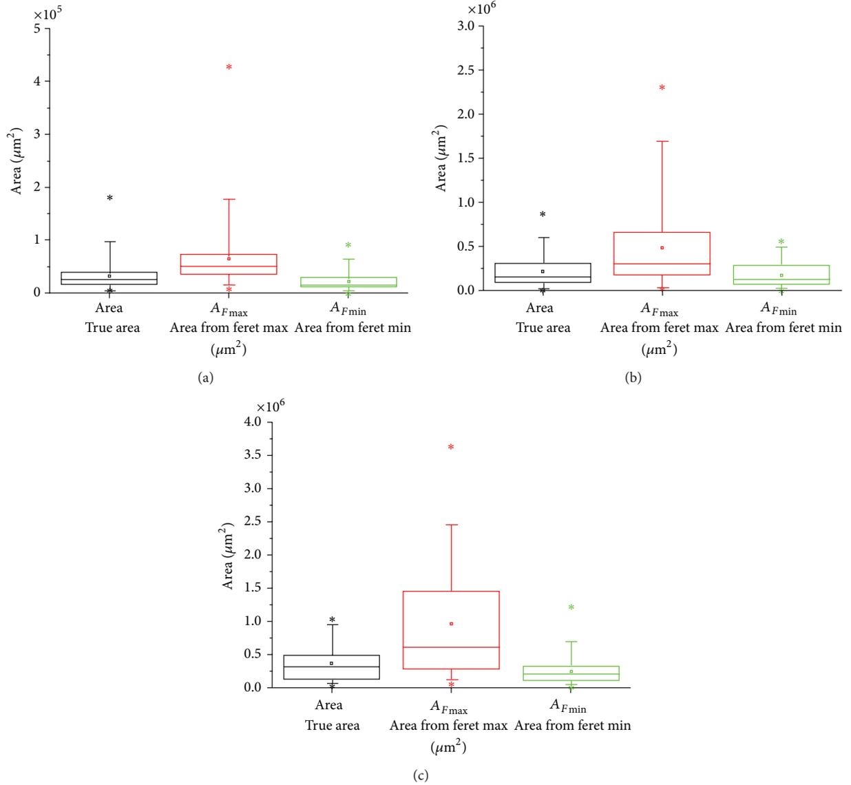
FIGURE 8: Comparison between the true fiber area directly measured by image analysis and the areas calculated assuming circular cross-sections: (a) *E. elatior*, (b) *C. comosus*, and (c) *H. bihai* fibers.
