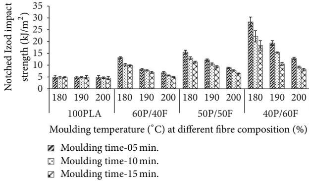
FIGURE 2: Effect of process variables on the notched Izod impact strength.
