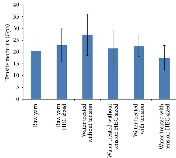
FIGURE 2: Tensile modulus of single jute fibre (error bars indicate standard deviation).
