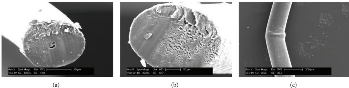
FIGURE 12: SEM images showing different features of cattle hair (with and without a hole in the middle, kink bands).
