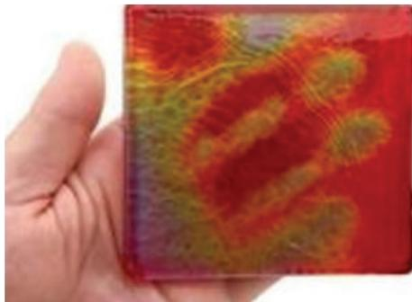
FIGURE 6: Smart electrospun nanofibre membranes produced PNI-PAM [67].
