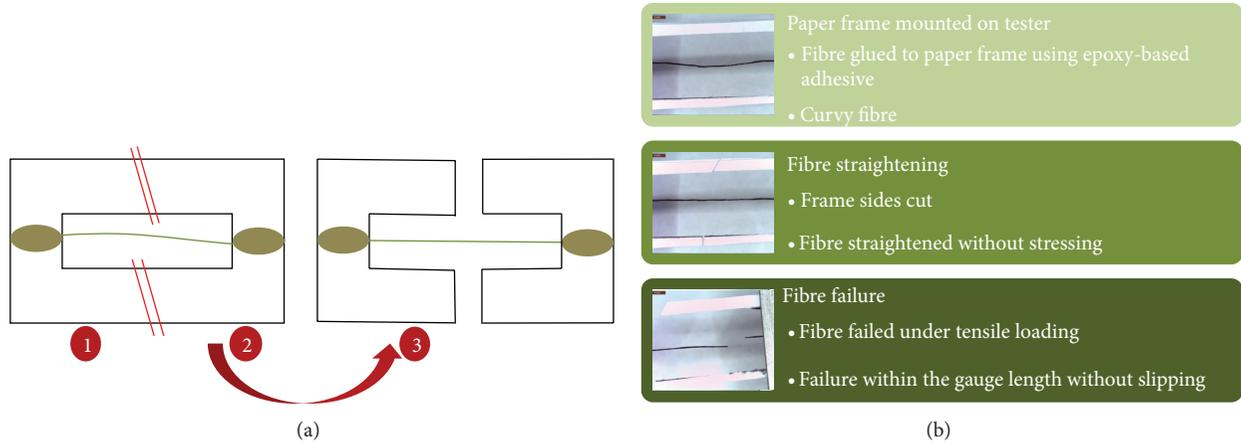
FIGURE 1: Schematic presentation showing preparing the fibre for tensile testing and optical microscope images taken during the process.
