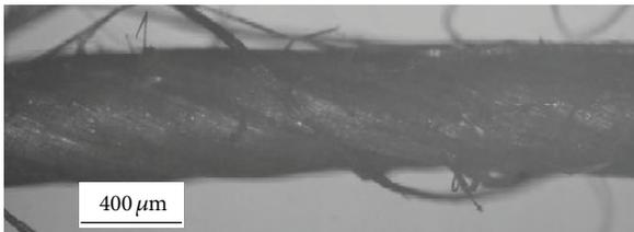
FIGURE 4: Water-treated yarn without tension and HEC sized.
