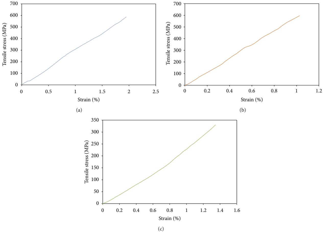
FIGURE 6: Representative curves for tensile behaviour of (a) hemp single fibres, (b) flax single fibres, and (c) Jute single fibres.
