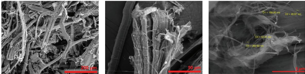
FIGURE 2: Ultrasonic-treated hemp fibers after steam explosion (F SE WA US).
