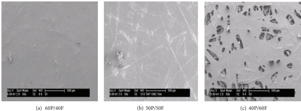
FIGURE 7: SEM micrographs of the biocomposite surfaces with different flax fibre content.
