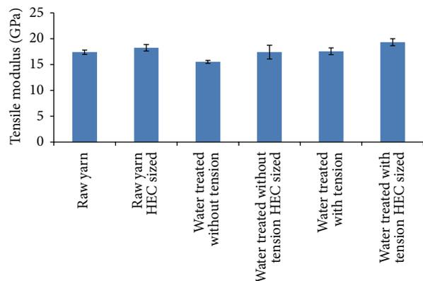
FIGURE 11: Tensile modulus of composites (error bars indicate standard deviation).
