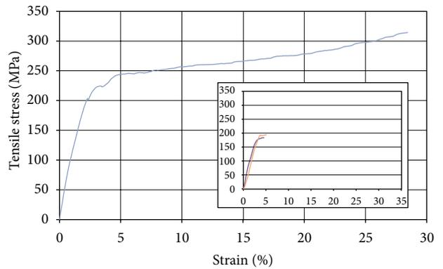
FIGURE 4: Representative curves for tensile behaviour of some of the tested cattle hair fibres with the inset showing samples with early premature failure.
