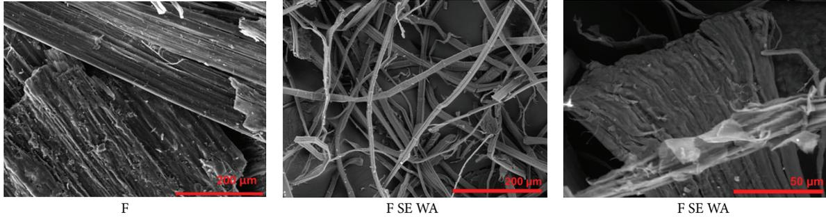
FIGURE 1: Untreated and steam-exploded hemp fibers.
