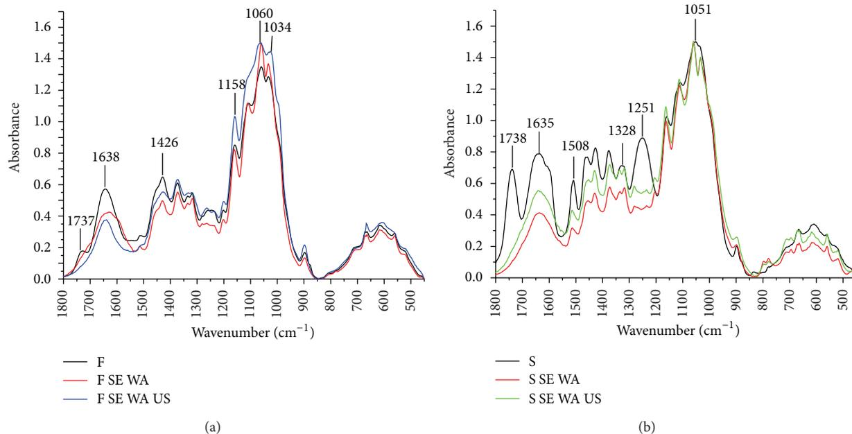
FIGURE 5: FTIR spectra of untreated, steam-exploded, and HIUS-treated hemp fibres (F) and shives (S).
