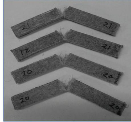
FIGURE 3: Photograph of the impact tested biocomposite samples with 60 wt% flax fibre.
