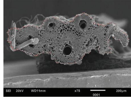
FIGURE 2: Manual outline of the fiber's perimeter. Example for a *C. comosus* fiber.
