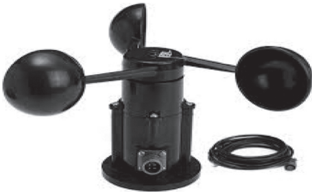
FIGURE 9: Wind speed measure sensor.
