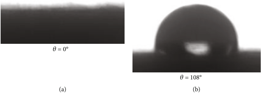
FIGURE 6: Contact angle of unsized and AKD-sized papers (contact time = 5 s): (a) Sample C, no AKD added; (b) Sample A2, 0.2% AKD added.
