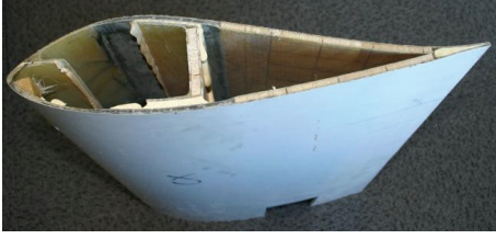
FIGURE 2: Cross section view of CX-100.
