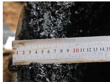
FIGURE 10: Wax deposition at the outlet of the first interval of the long-term unpigged pipeline (about 80 mm).
