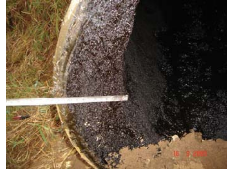
FIGURE 9: Maximum wax deposition of the first interval of the long-term unpigged pipeline (about 110 mm).
