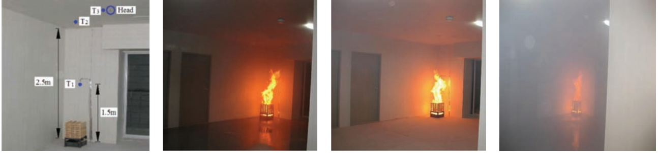
FIGURE 6: Fire ignition and suppression sequence during the actual fire test.
