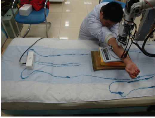
FIGURE 2: Experimental setup for measuring mechanical properties of living tissue.
