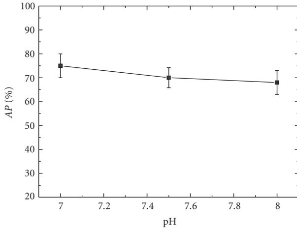
FIGURE 7: pH effect on adsorption ampicillin at 30°C.
