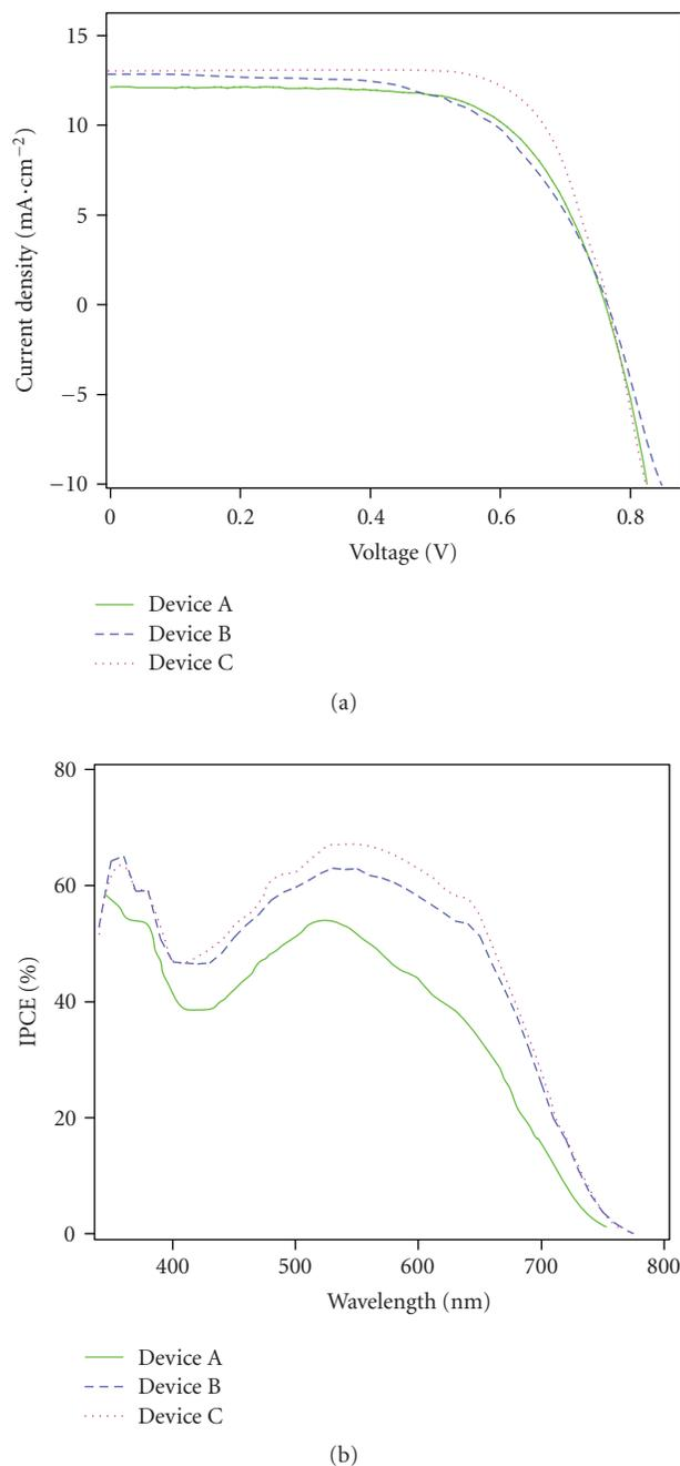
FIGURE 2: (a) Photocurrent intensity-voltage characteristics for devices A, B, and C, measured at 1 sun (1000 W  $\cdot$  m<sup>-2</sup>), AM 1.5 global sunlight illumination. (b) Photocurrent action spectra of the same devices.
