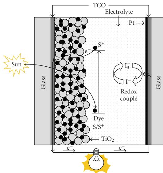
FIGURE 1: Schematic representation of a dye-sensitized solar cell.
