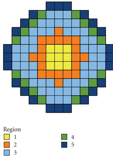
FIGURE 2: Radial cross-section of the NEK core.
