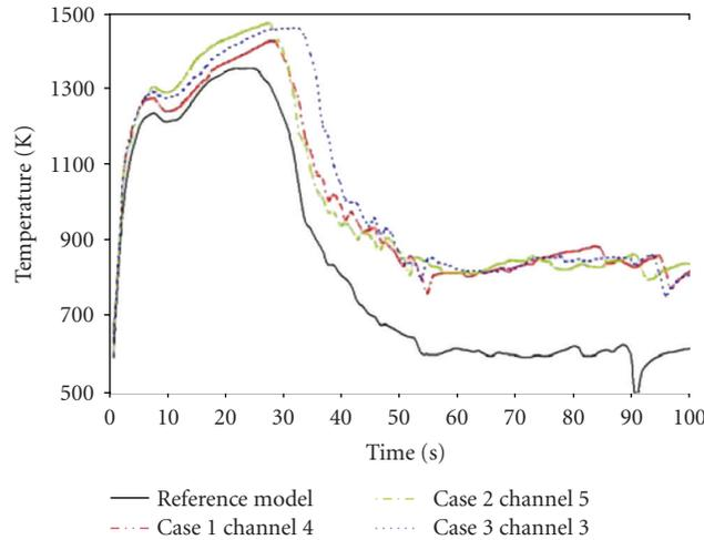
FIGURE 15: Maximum fuel bundle cladding temperatures for a CANDU-6 Inlet manifold break analysis for different break locations.
