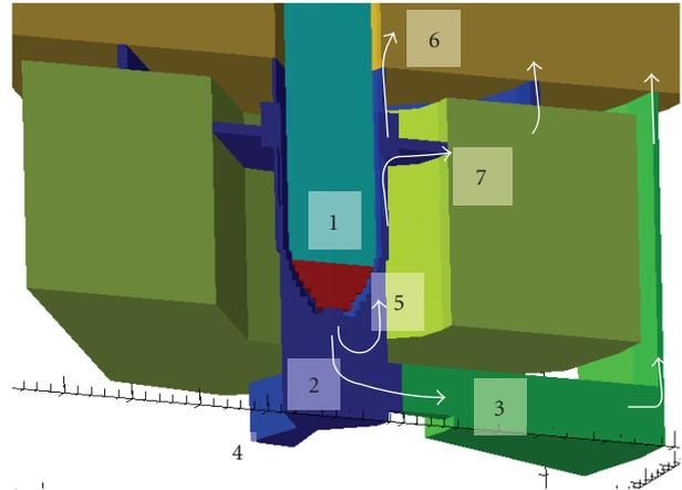
FIGURE 1: Example of 3D test calculation geometry with a fine mesh, showing the main volumes and flow paths, for the DISCO-F geometry. 1 reactor pressure vessel, 2 reactor cavity, 3 reactor pit access, 4 pit niche, 5 annular space, 6 exit to containment, 7 exit to subcompartments.
