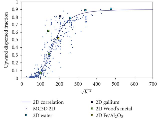
FIGURE 12: All calculations versus proposed correlation for 2D case, and available 2D experimental data.
