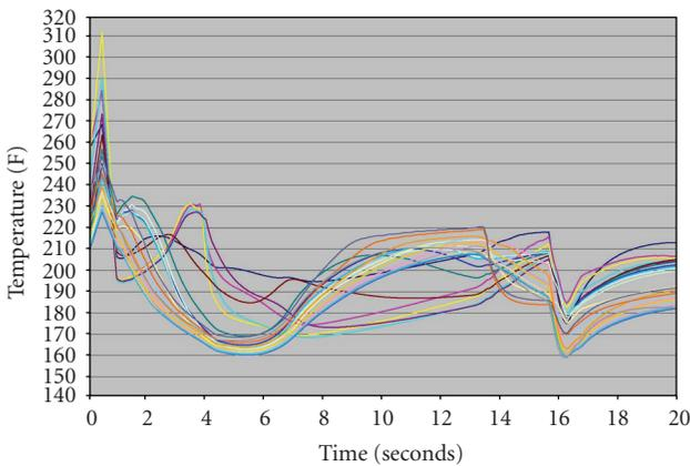
FIGURE 6: Example of RELAP/SCDAPSIM-calculated fuel plate centerline temperatures for the 24 fuel plates in MURR for a cold leg large break transient.
