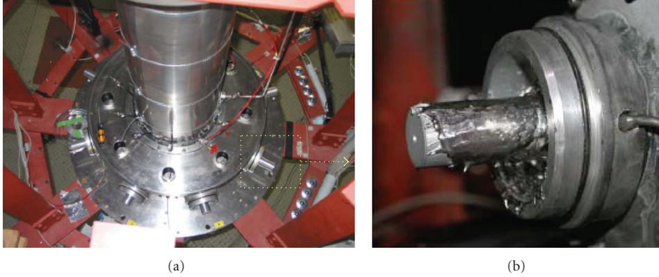
FIGURE 2: DISCO-F experimental setup. (a) View from above at the cavity exit holes and the main cooling line stubs during assembly of the test rig. (b) Close view of exit around one cooling line after a test with liquid metal.
