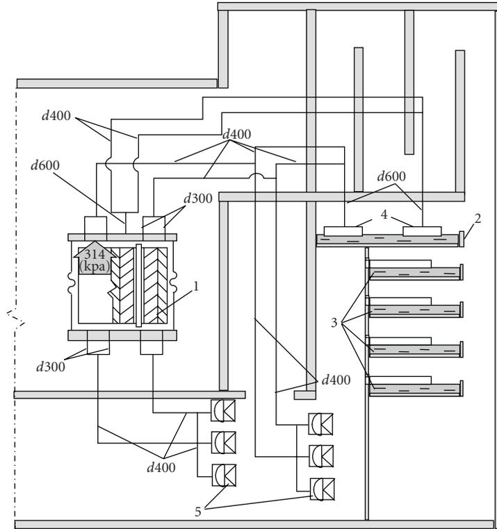
FIGURE 5: Simplified schematic of the reactor cavity venting system: (1) reactor, (2) the fifth ALS suppression pool, (3) suppression pools 1–4, (4) steam distribution devices, and (5) membrane safety devices (350 mm diameter)
