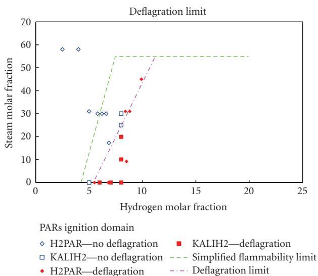
FIGURE 9: Ignition of SIEMENS PARs.
