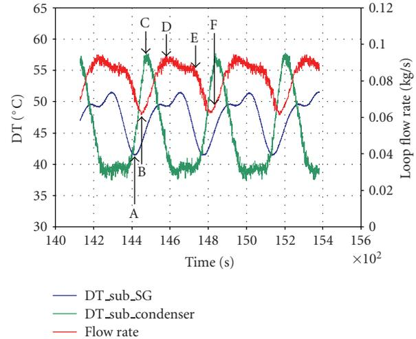
FIGURE 9: Low-frequency oscillations: steam generator inlet subcooling, pool condenser outlet subcooling, and loop flowrate as a function of time (Data obtained with power = 23 kW – FR = 0.79 – with heat losses compensation).
