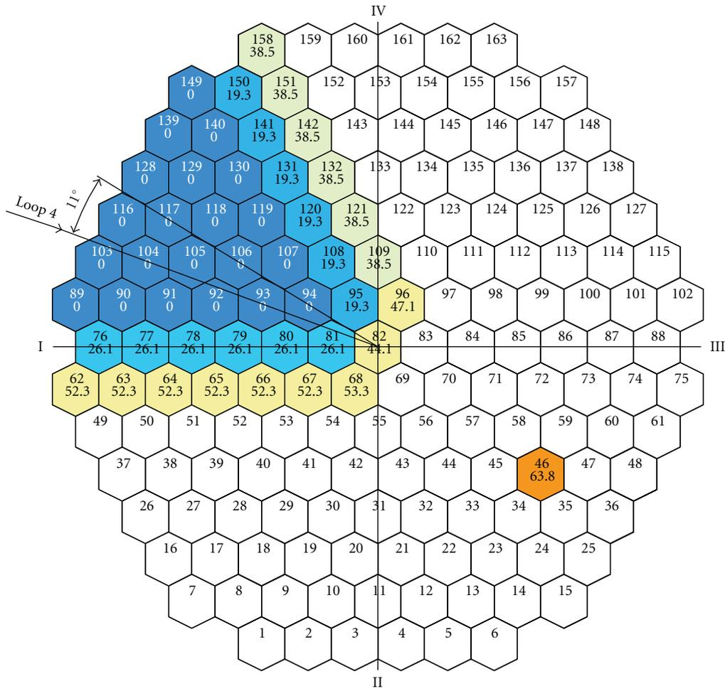
FIGURE 10: MSLB Scenario 2 with stuck rods no. 117 and no. 140: CATHARE 12-sector calculated angular turn of loop no. 4 flow centre.
