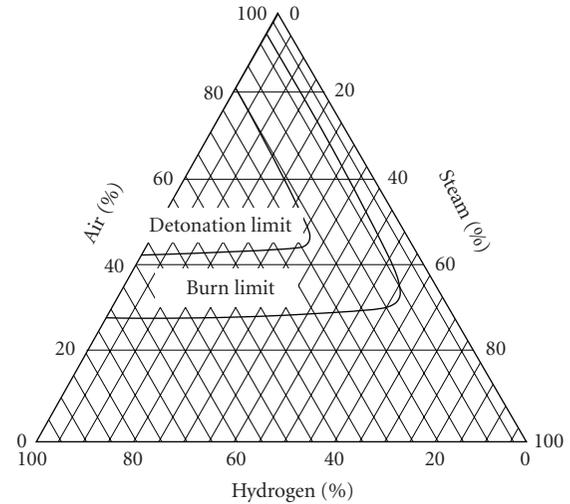
FIGURE 1: Shapiro diagram for hydrogen-air-steam mixtures.
