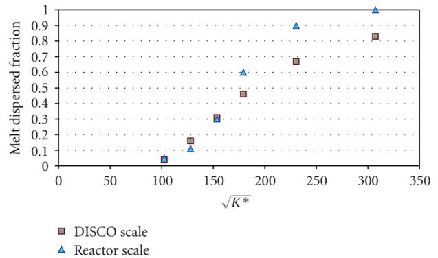
FIGURE 15: Impact of scaling regarding the upward fuel dispersion estimated with 2D MC3D calculations in cold conditions and heavy metal (Wood's metal).
