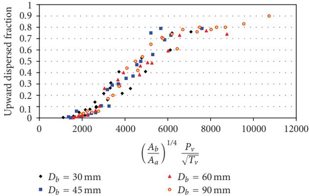
FIGURE 11: Impact of vessel gas temperature and break diameter on the calculated upward dispersed fraction (all other parameters identical).
