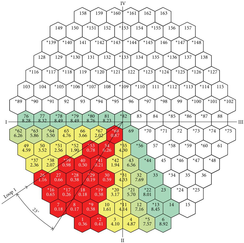
FIGURE 7: CATHARE 24-sector vessel model: angular turn of the loop no. 1 flow centre.
