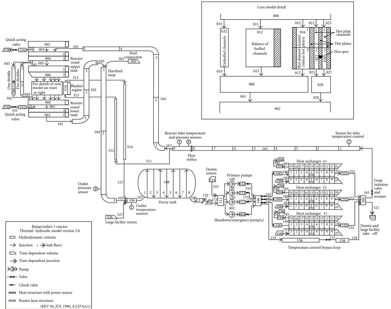
FIGURE 5: RELAP/SCDAPSIM nodalization of the SAFARI cooling system.
