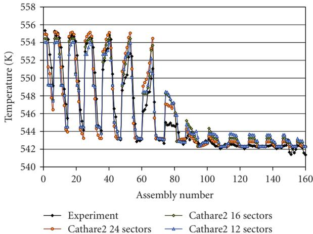
FIGURE 4: Kozloduy-6 flow mixing test: assembly by assembly core inlet temperatures.
