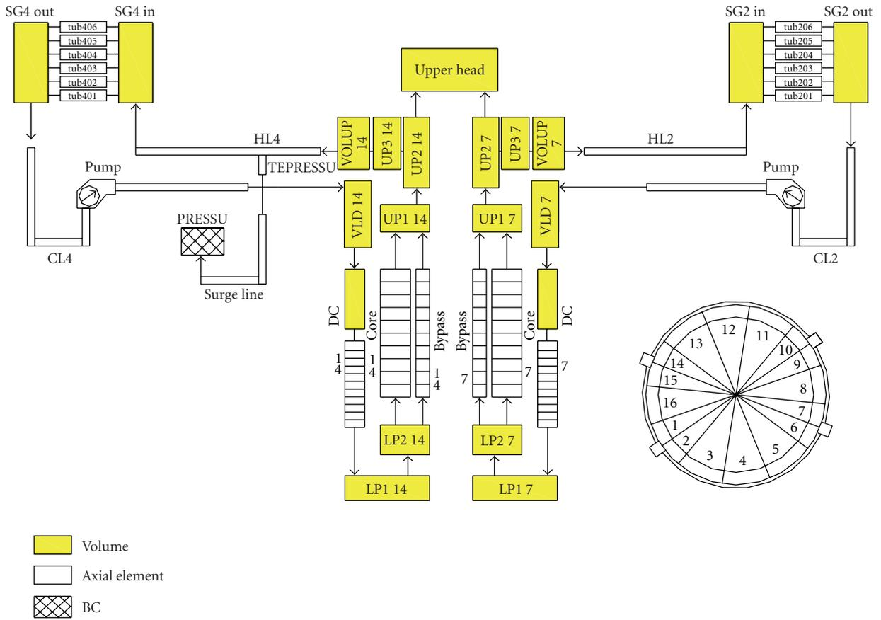
FIGURE 2: Primary circuit nodalization scheme (2 of 16 vessel channels are shown).
