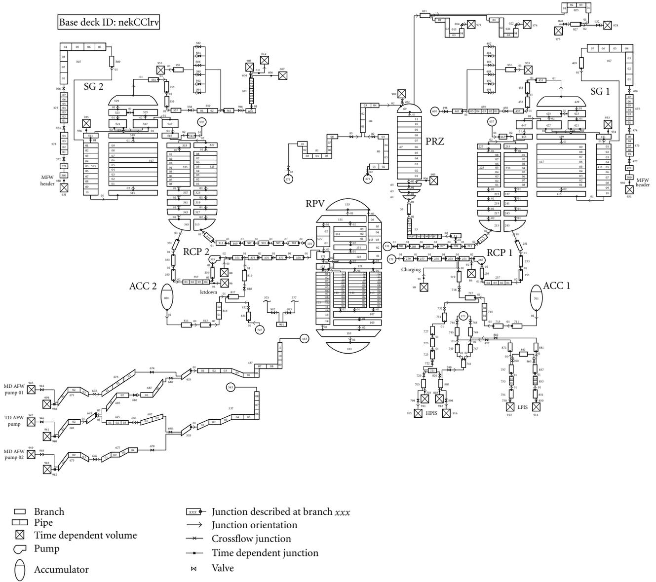
FIGURE 1: NEK RELAP5/Mod3.3 nodalization scheme.
