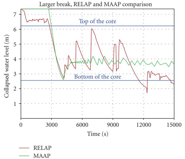
FIGURE 16: Collapsed water level in the reactor vessel, Group 2.
