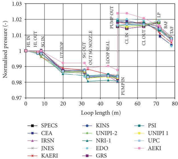
FIGURE 4: Normalized pressure curve along the loop.
