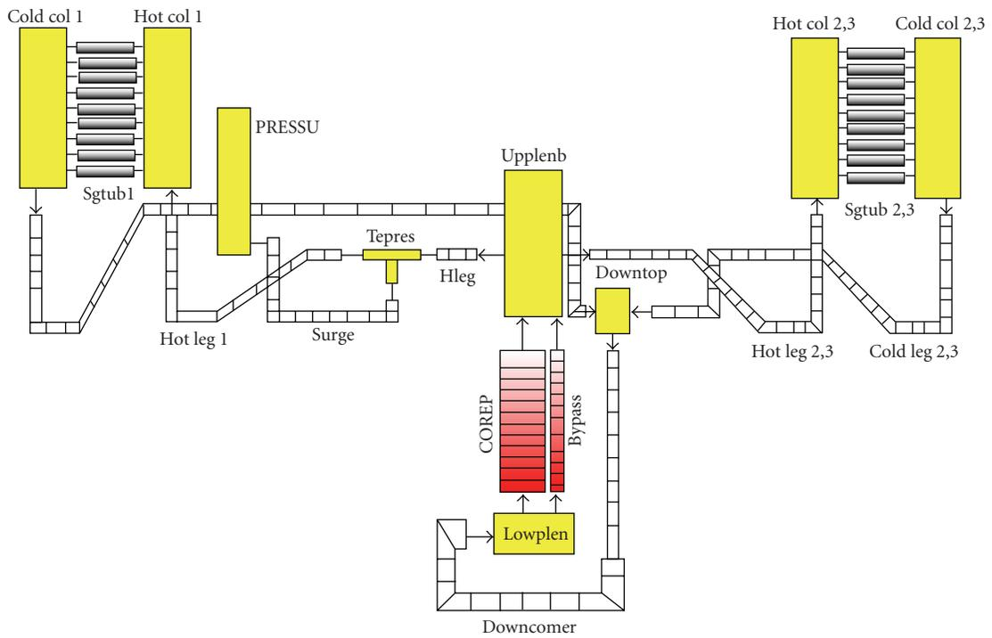
FIGURE 3: CATHARE nodalization of the PACTEL primary circuit.
