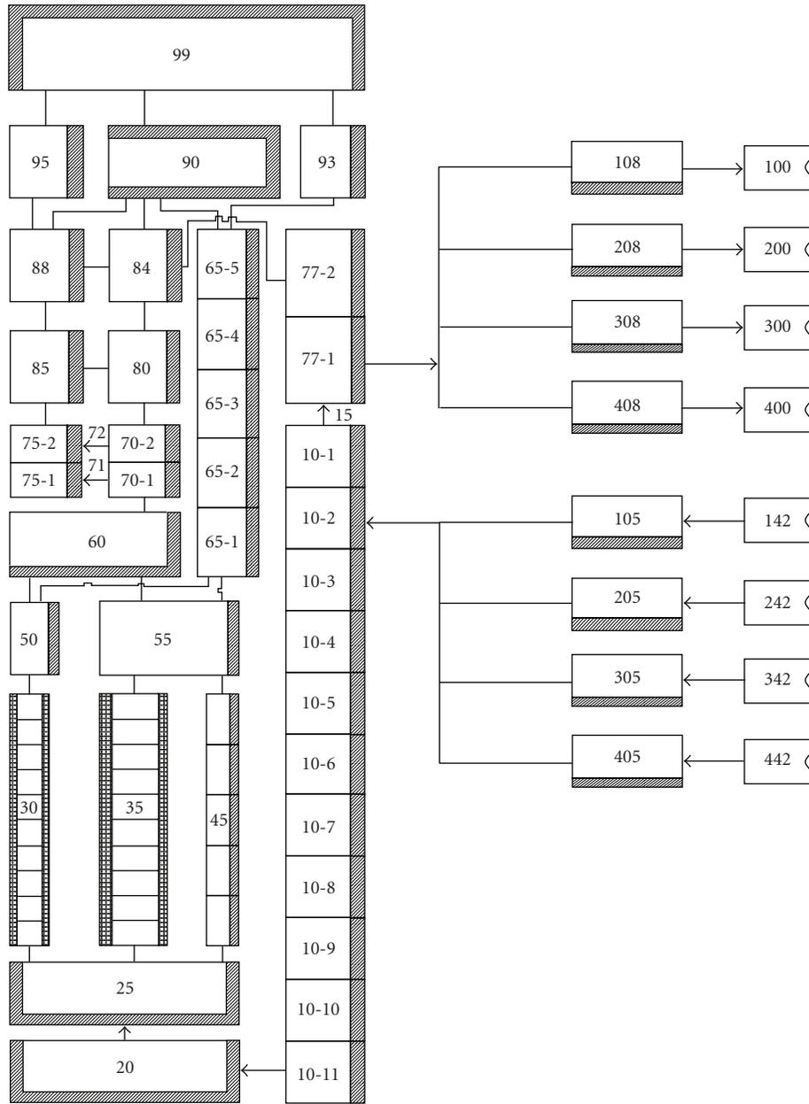
FIGURE 17: Representative vessel input nodalization for VVER-1000 for transients not including the possibility of loss of core geometry.
