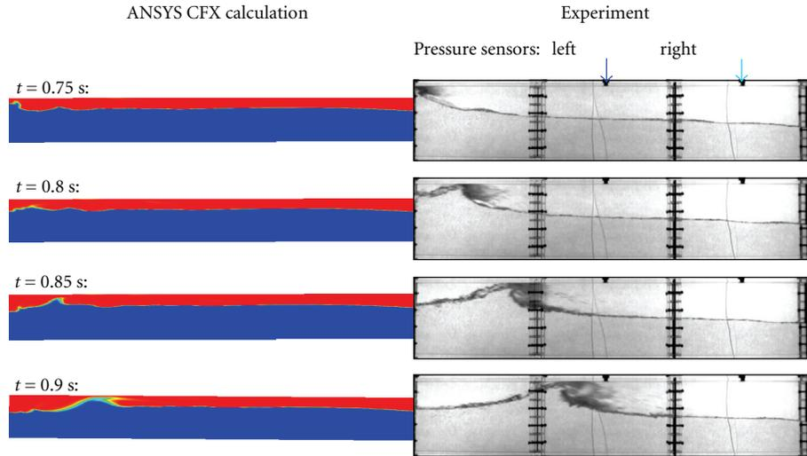
FIGURE 5: Comparative picture sequence of the recalculated slug.
