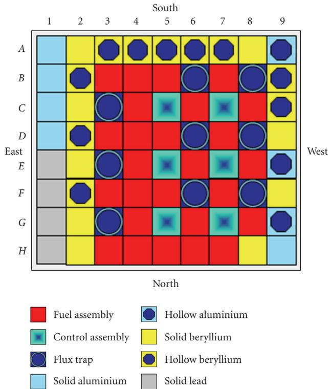
FIGURE 1: SAFARI reactor core configuration.
