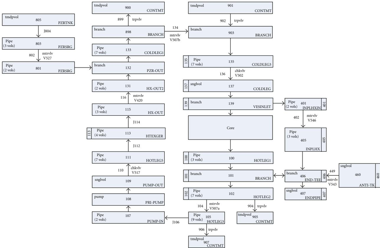
FIGURE 2: MURR RELAP/SCDAPSIM nodalization of the MURR pressurized primary cooling system.
