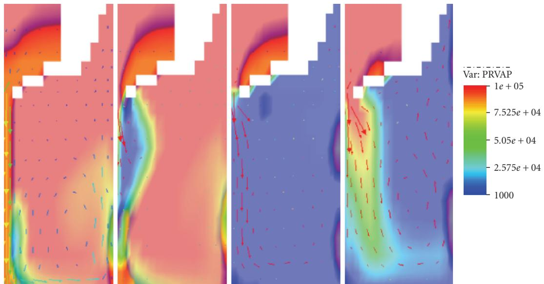
FIGURE 9: Visualization of vapour partial pressure during the phase of melt ejection (same calculation as in Figure 6). Legend: vapour partial pressure (Pa), see also Figure 6 for continuous melt volume fraction and drop velocity. Frames at times as for Figure 8:  $t = 0.08, 0.09, 0.15,$  and  $0.3$  second.
