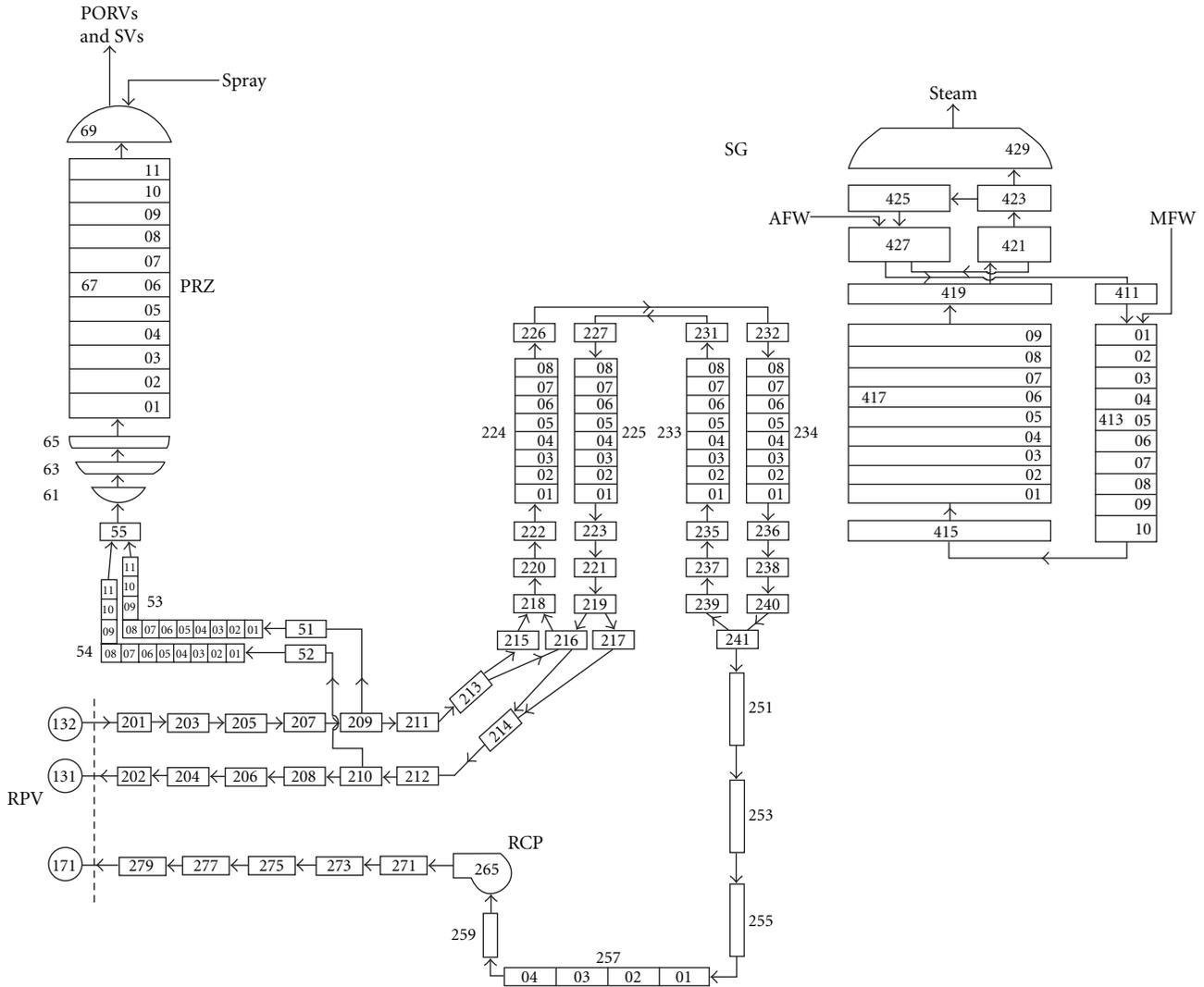
FIGURE 3: RELAP5/SCDAPSIM nodalization for modelling natural circulation.
