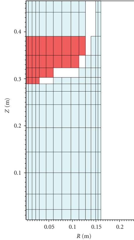
FIGURE 10: View of the grid used for the evaluation of correlation with MC3D (pit region only, white zone : solid structure, red : corium pool).
