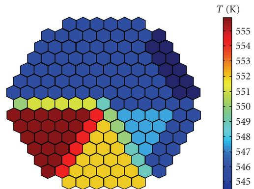
FIGURE 17: Predicted coolant temperature at core outlet at final state (1800 seconds).
