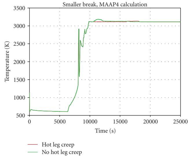
FIGURE 6: Core maximum temperature, MAAP4 calculation, Group 1.
