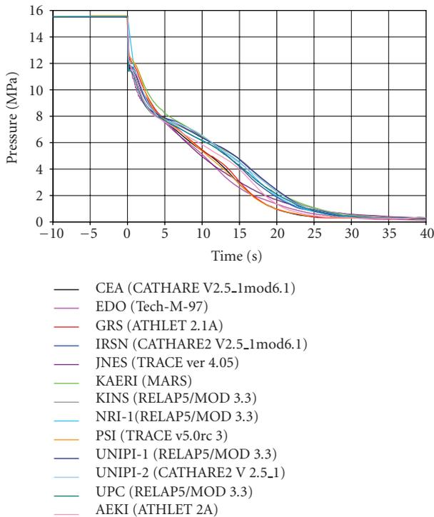
FIGURE 5: Time trends of intact loop 1 pressure in hot leg.
