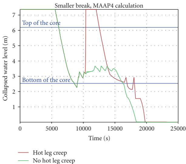
FIGURE 5: Collapsed water level in the reactor vessel, MAAP4 calculation, Group 1.
