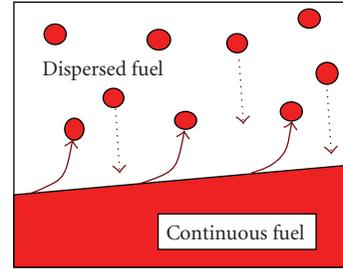
FIGURE 3: Connections between the continuous and discontinuous fuel fields. Plain arrows: fragmentation; dashed arrows: coalescence towards continuous fuel.
