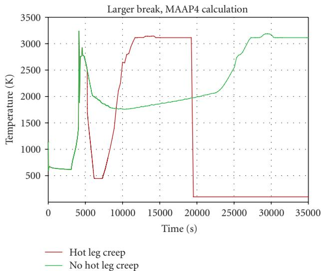
FIGURE 14: Core maximum temperature, MAAP4 calculation, Group 2.
