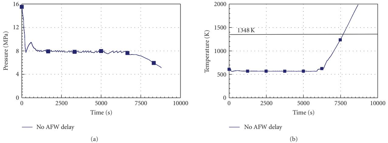
FIGURE 3: Scenario with AFW available: (a) RCS pressure, (b) core cladding temperature.
