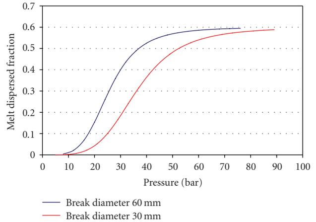
FIGURE 14: Application of correlation (14) to a case with corium as fuel, and vapor at 550 K in vessel for two break diameters, at the scale of DISCO tests (1/16th).
