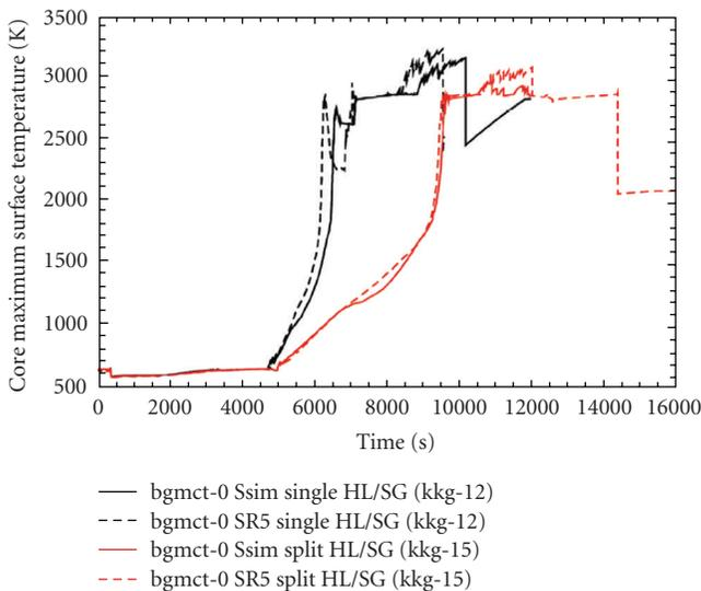
FIGURE 12: Example of RELAP/SCDAPSIM and RELAP/SCDAPSIM-calculated results for peak core temperature for single and split hot leg model.
