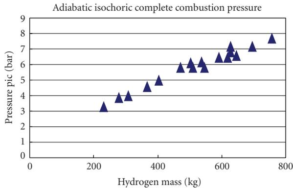
FIGURE 8: PAICC pressure versus hydrogen mass.
