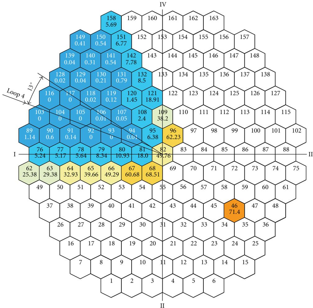
FIGURE 11: MSLB Scenario 2 with stuck rods no. 117 and no. 140. CATHARE 24-sector calculated angular turn of loop no. 4 flow centre.
