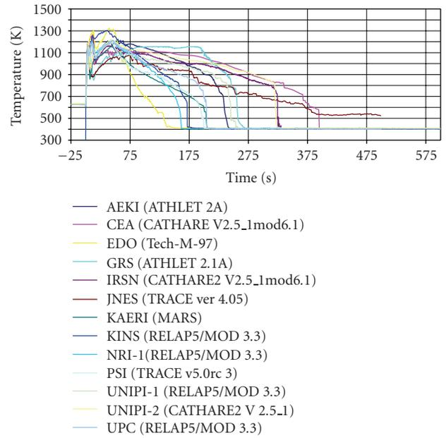
FIGURE 10: Time trends of maximum cladding temperature.
