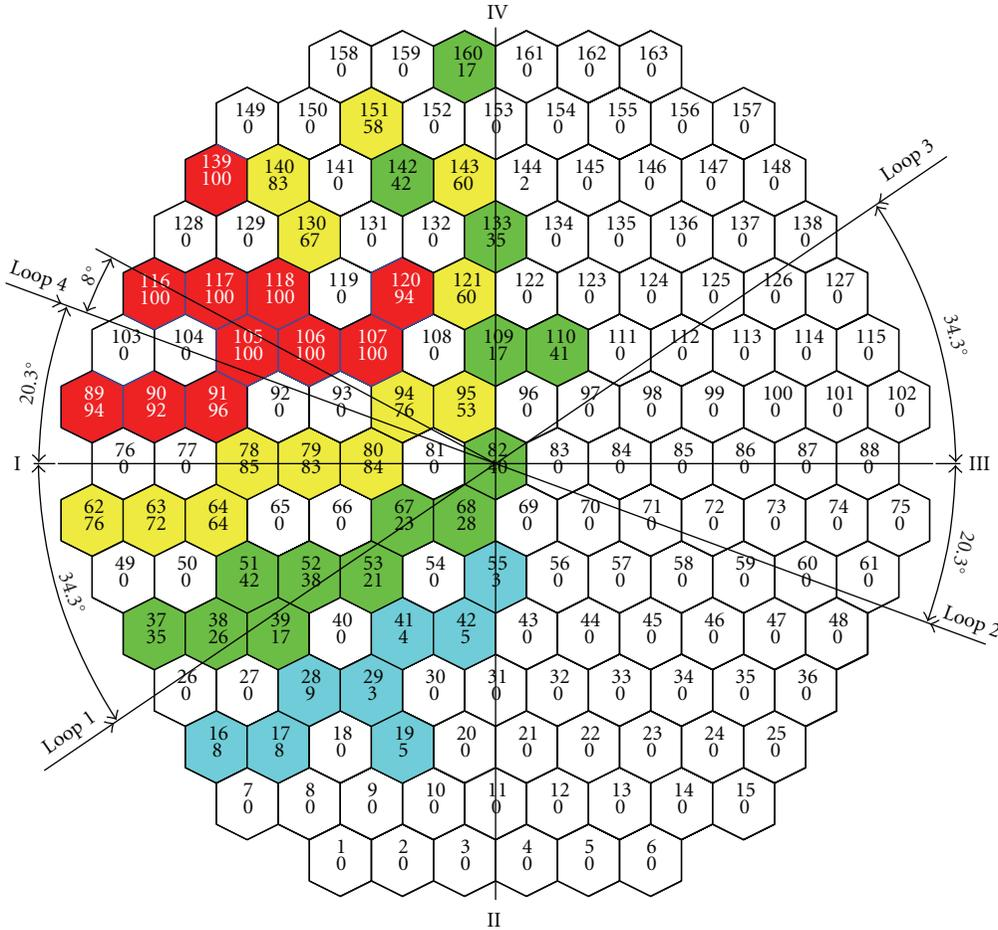
FIGURE 9: Kozloduy-6 vessel mixing experiment: assembly outlet data for loop-to-assembly mixing coefficients, and zone of minimal mixing and angular turn of the flow centre for loop no. 4.
