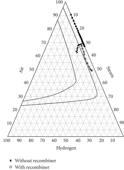
FIGURE 6: Effect of PARs on gas mixture flammability (with stars: gas composition without PARs; with circle: gas composition with PARs).
