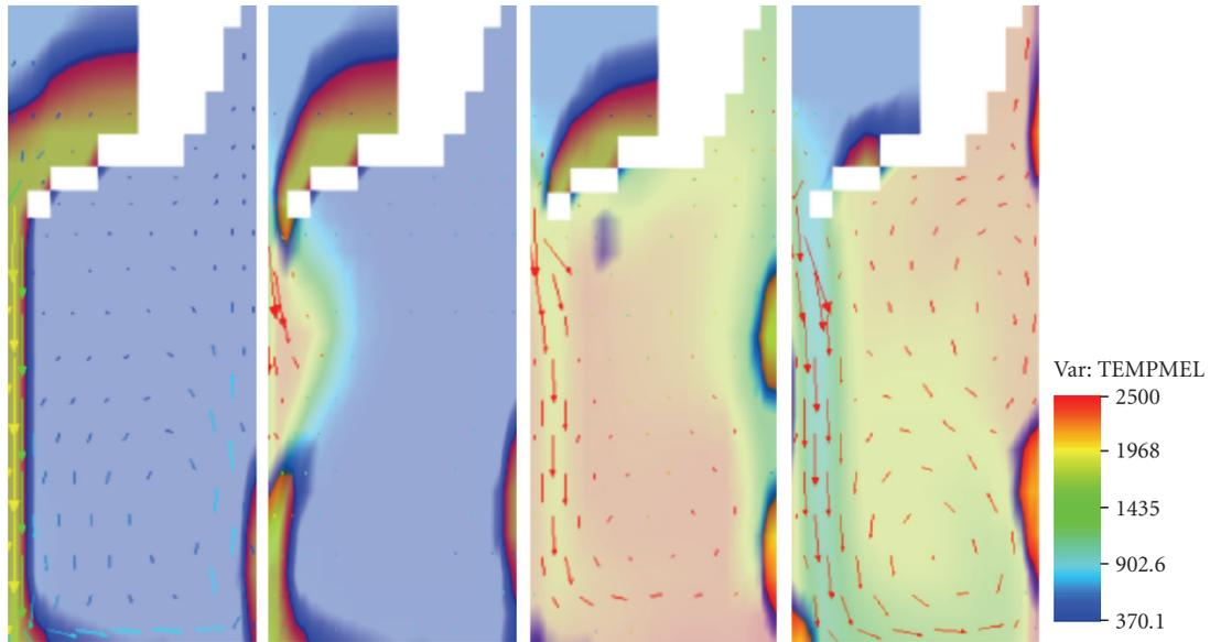
FIGURE 8: Visualization of gas temperature during the phase of melt ejection (same calculation as in Figure 6). Legend: gas temperature (K), see also Figure 6 for continuous melt volume fraction and drop velocity. Frames at times  $t = 0.08, 0.09, 0.15,$  and  $0.3$  second.
