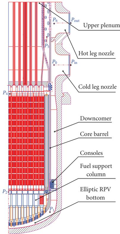
FIGURE 1: VVER-1000 reactor pressure vessel and internals.
