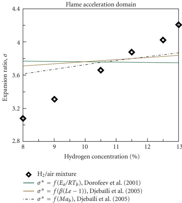
FIGURE 2: Critical value  $\sigma^*$  as a function of hydrogen concentration.
