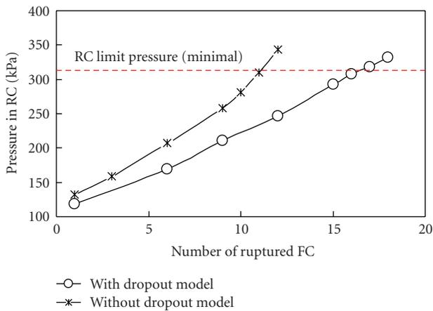
FIGURE 6: Pressure in the reactor cavity as a function of a number of ruptured fuel channels.
