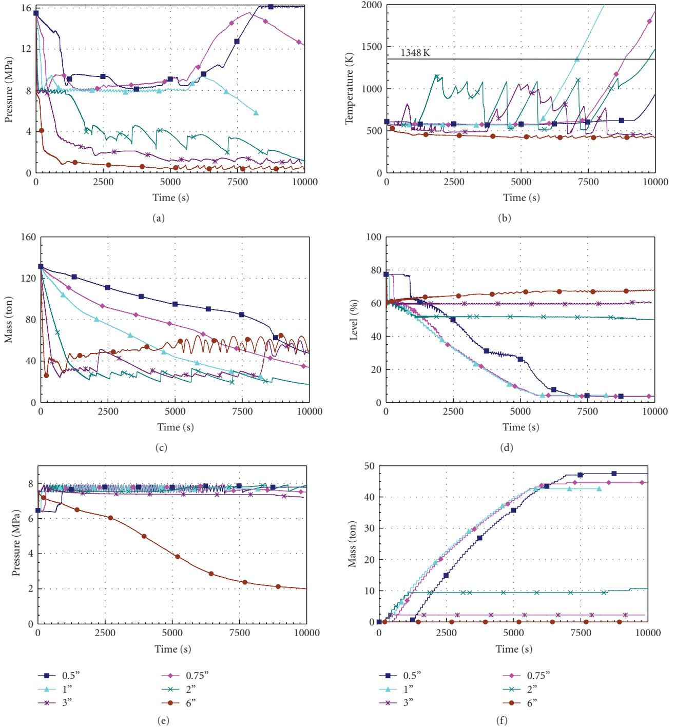
FIGURE 2: Calculated results for spectrum of break sizes: (a) RCS pressure, (b) core cladding temperature, (c) RCS mass inventory, (d) SG no. 1 wide range level, (e) SG no. 1 pressure, (f) mass discharged through SG no. 1 PORV.
