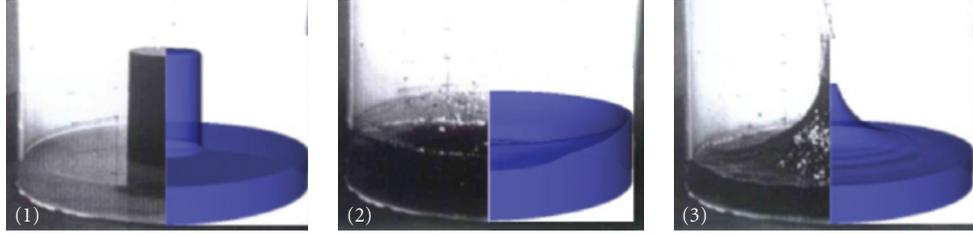
FIGURE 4: Continuous field slosh test computed by the MC3D code in 2D with a VOF-PLIC approach (the 3D effect is a result of image processing). Each image compares the code visualisation (on the right) with the experiments [9] using water (on the left): (1) initial state of a water cylinder immersed in a shallow basin of water; (2) first maximum at the wall, (3) maximum at the centre after two sloshing movements.
