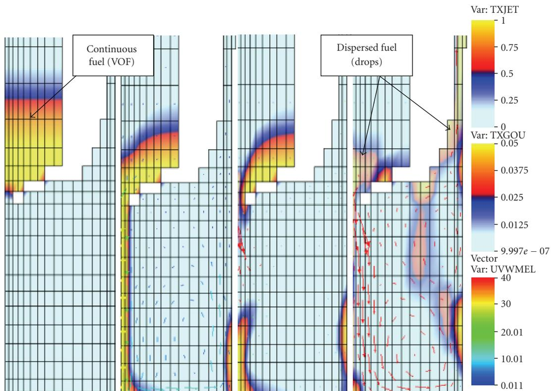
FIGURE 6: Visualization of melt ejection fragmentation and upward dispersion in a typical simulation of DISCO integral test ( $P_v = 19$  bar,  $D_b = 30$  mm,  $\text{Al}_2\text{O}_3\text{-Fe}$  thermite at 2500 K, vessel gas: vapour). Legend: top: continuous fuel field volume fraction, middle: fuel drop volume fraction, bottom: drop velocity (m/s). Frames at times  $t = 0, 0.08, 0.09$ , and  $0.3$  seconds.
