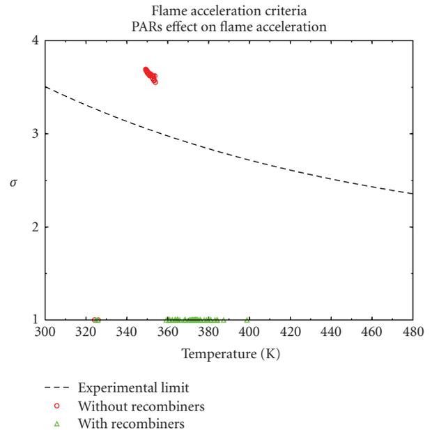
FIGURE 7: PARs effect on Flame acceleration (in red: gas composition without PARs; in green: gas composition with PARs).
