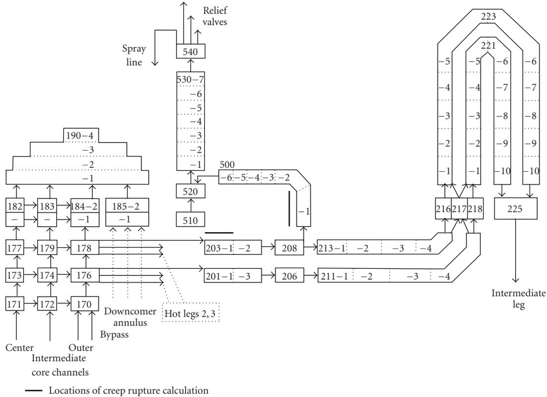
FIGURE 11: Gösgen split hot leg nodalization used for RELAP/SDAPSIM and SCDAP/RELAP5.
