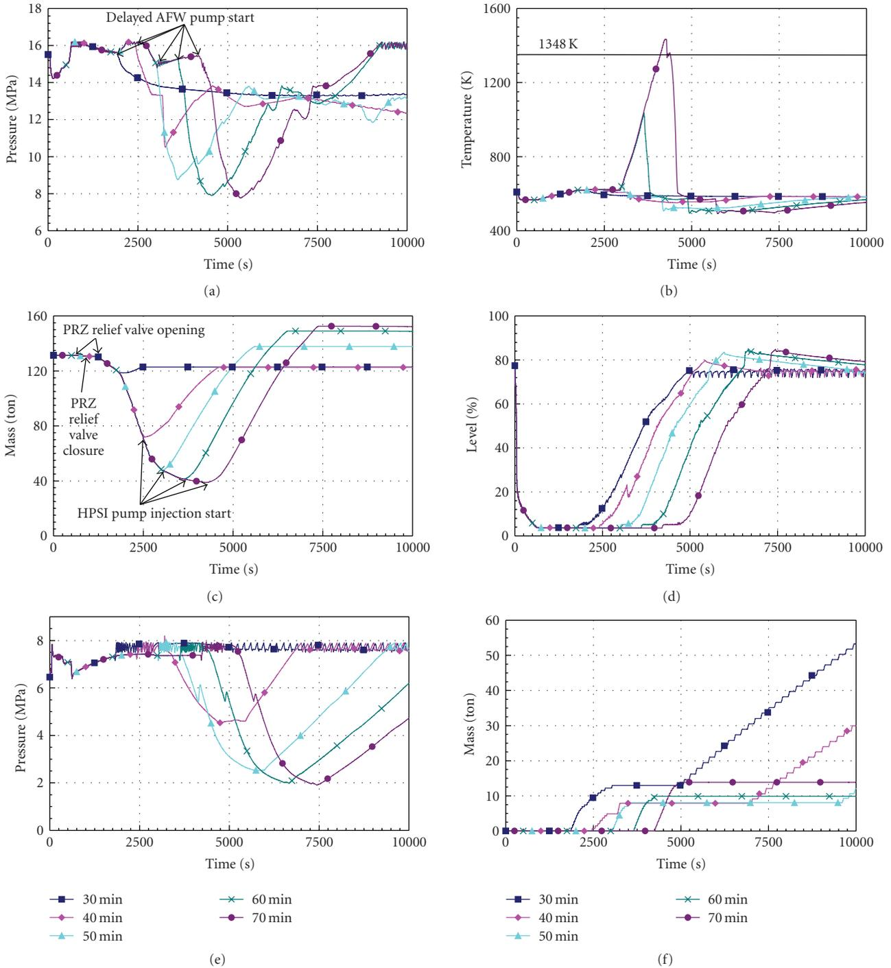
FIGURE 5: LOFW transient: (a) RCS pressure, (b) core cladding temperature, (c) RCS mass inventory, (d) SG no. 1 wide range level, (e) SG no. 1 pressure, (f) mass discharged through SG no. 1 PORV.
