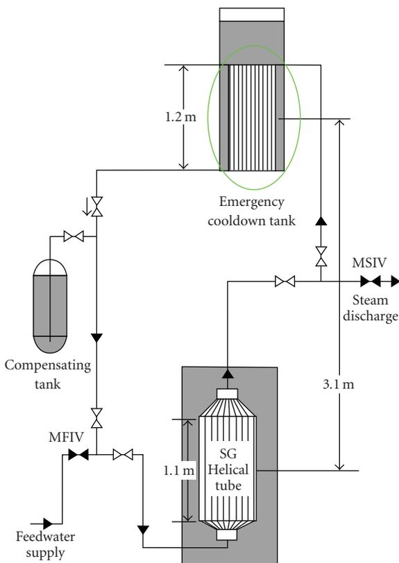
FIGURE 5: PRHR condenser of the SMART.
