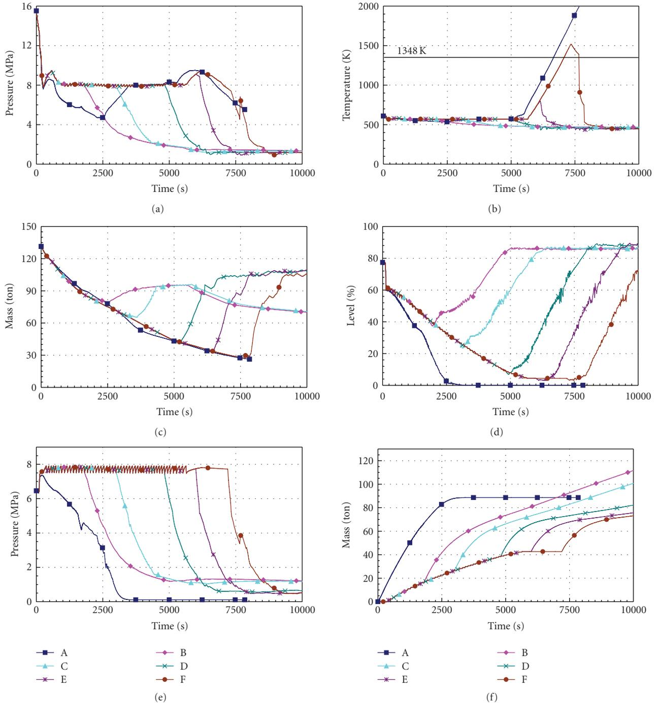
FIGURE 4: 2.54 cm break scenarios with two operator actions: (a) RCS pressure, (b) core cladding temperature, (c) RCS mass inventory, (d) SG no. 1 wide range level, (e) SG no. 1 pressure, (f) mass discharged through SG no. 1 PORV.
