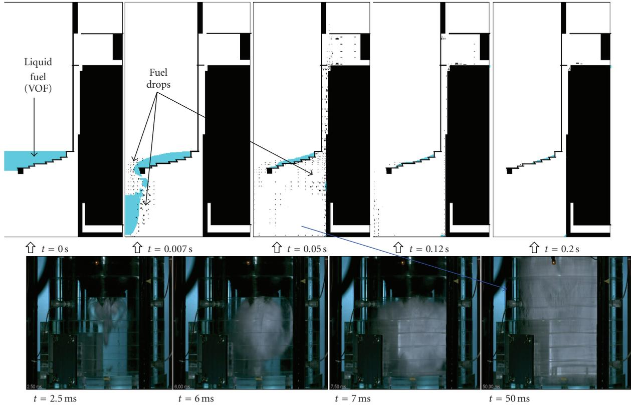
FIGURE 7: Pictures of the pit during test F07 (bottom) compared with a visualization of flow computed with MC3D (top).
