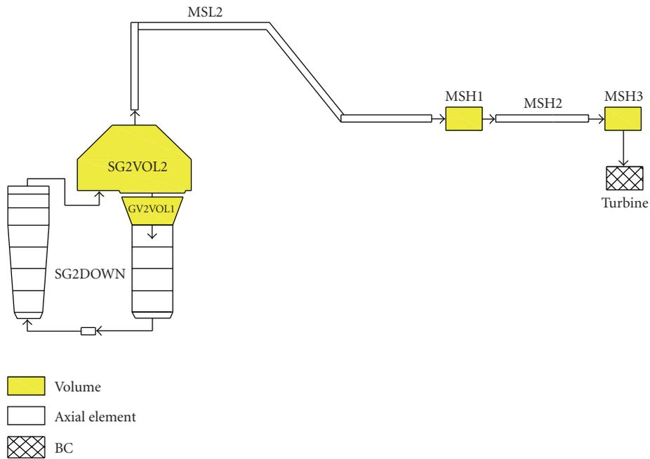
FIGURE 3: Secondary circuit nodalization scheme (SG-2 and steam line 2 are shown).
