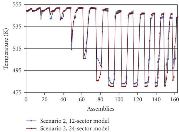
FIGURE 8: Snapshot for MSLB Scenario 2 at highest return to power: assembly by assembly core inlet temperatures for different angular meshes.
