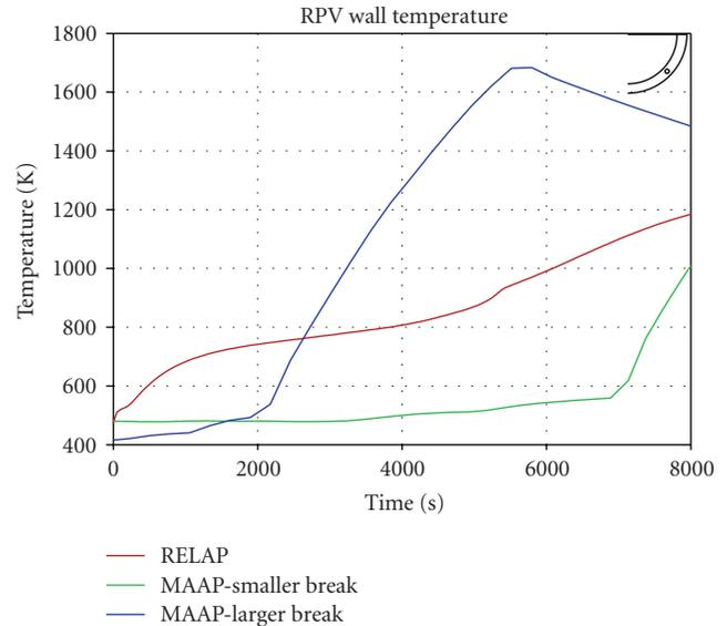
FIGURE 19: Temperature of the wall of the RPV lower head after relocation of molten material (the red dot on the figure in the upper right corner represents the position at the RPV wall where the temperature was calculated).
