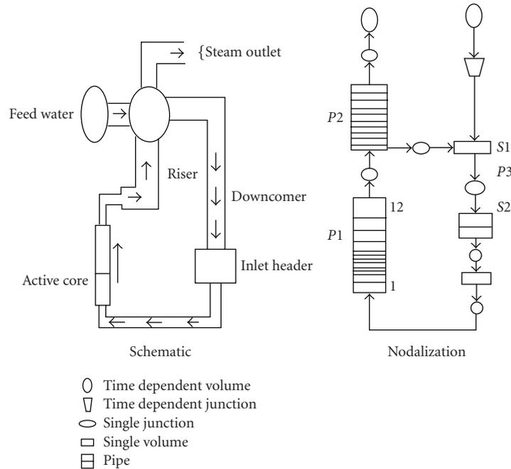
FIGURE 22: Example of university applications—natural circulation boiling water reactor applications by IIT-Guwahati.
