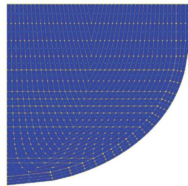
FIGURE 11: COUPLE model of the NEK RPV lower head.
