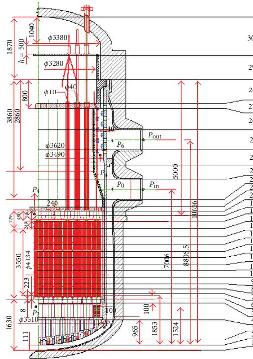
FIGURE 7: TRACE axial nodalization of the RPV.
