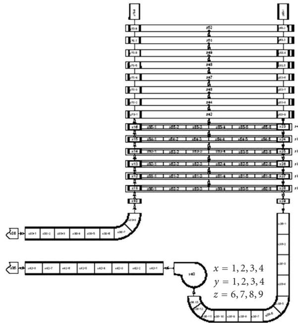
FIGURE 18: Representative loop input nodalization for VVER-1000.
