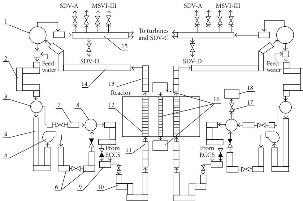
FIGURE 19: Representative RCS nodalization for RBMK.
