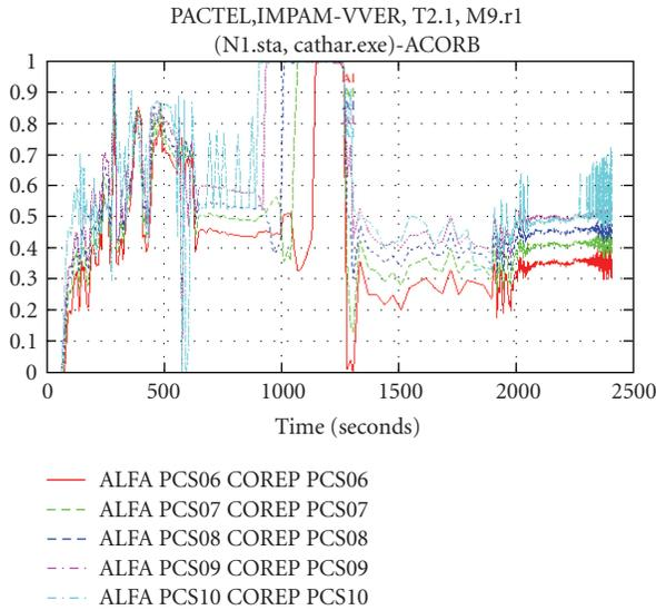
FIGURE 6: Void fractions (core upper half part).
