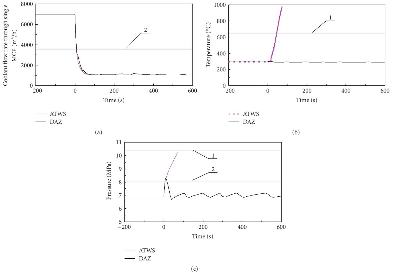
FIGURE 3: Analysis of loss of preferred electrical power supply and simultaneous failure of design reactor shutdown system, when DAZ system was installed: (a) coolant flow rate through one main circulation pump, (b) the peak fuel channel wall temperature in the high-power channel, (c) pressure behavior in drum separators, (1) acceptance criterion, and (2) set points of DAZ system activation (reactor shutdown).
