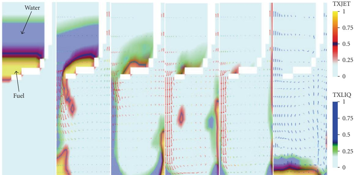
FIGURE 16: Example of calculation made with a situation where an important mass of saturated water is present in the vessel at the time of failure.  $P_v = 7$  bars, geometry as disco FH05 (see, e.g., Figure 6). Frames at times  $t = 0, 0.04, 0.12, 0.16, 0.3, 0.75$  seconds.
