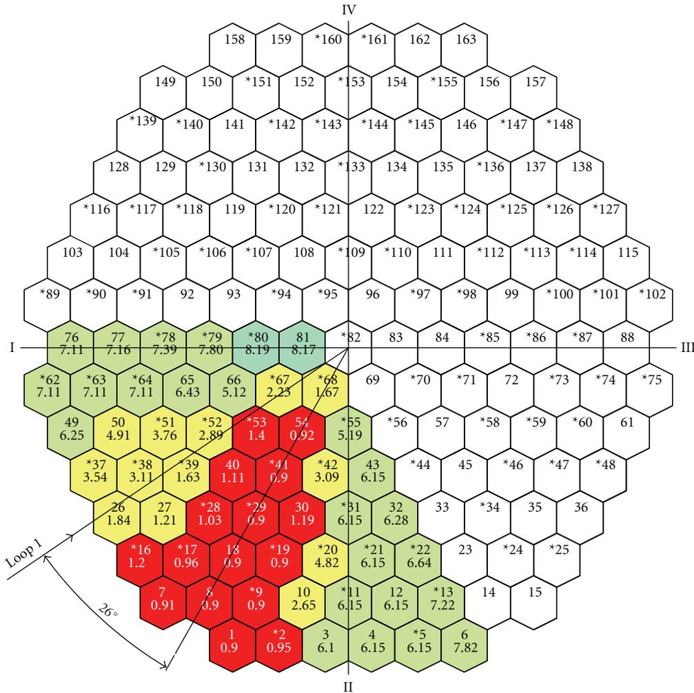
FIGURE 6: CATHARE 16-sector vessel model: angular turn of the loop no. 1 flow centre.
