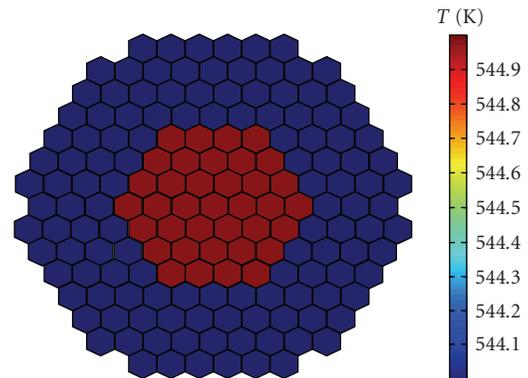
FIGURE 16: Predicted coolant temperature at the core outlet at initial state (0 second).
