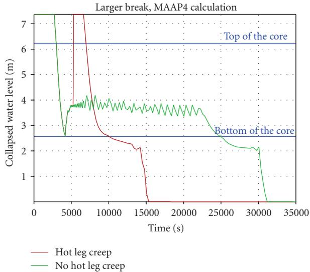
FIGURE 13: Collapsed water level in the reactor vessel, MAAP4 calculation, Group 2.
