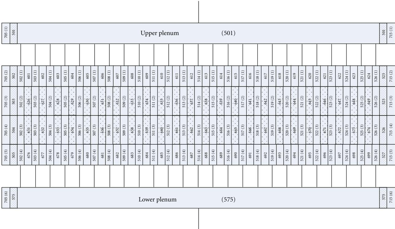
FIGURE 4: RELAP/SCDAPSIM nodalization of the MURR 24 fuel plate core.
