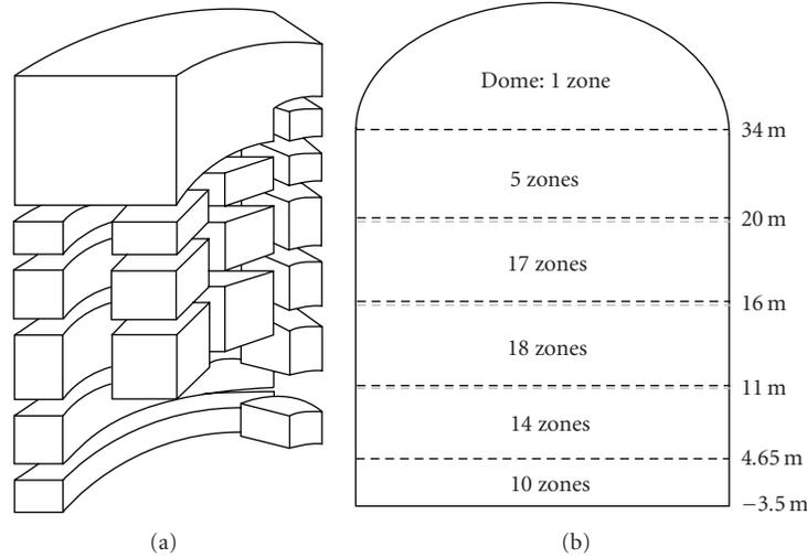
FIGURE 4: View of PWR 900 Astec nodalisation.
