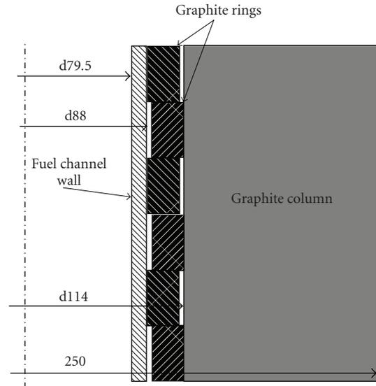
FIGURE 4: Fuel channel and graphite column interaction. All measurements are in millimeters.
