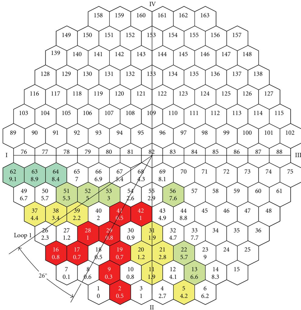
FIGURE 5: Plant data: estimated temperature differences (K) from cold leg no. 1 to the assembly inlets and angular turn of the loop no. 1 flow centre.
