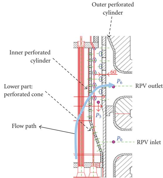
FIGURE 6: Vertical arrangement of the VVER-1000 primary components.
