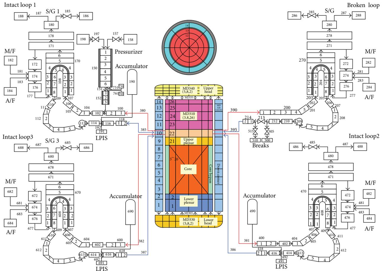
FIGURE 3: Example of 3-D MARS vessel nodalization scheme used by KAERI.
