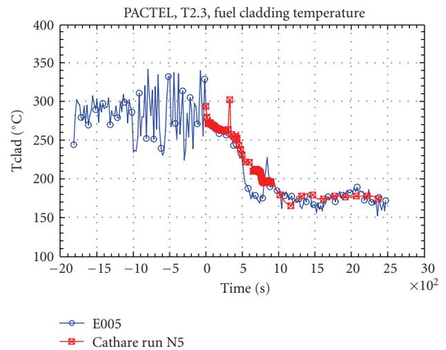
FIGURE 9: Fuel cladding temperature.
