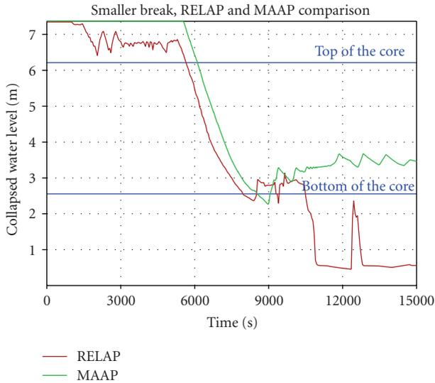
FIGURE 8: Collapsed water level in the reactor vessel, Group 1.
