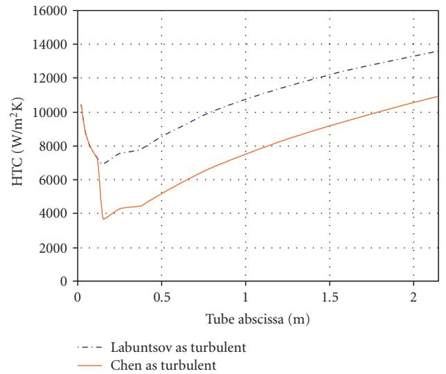
FIGURE 17: Condensation HTC along tube abscissa, according to film condensation theory ( $G = 61.5 \text{ kg/sm}^2$ ).
