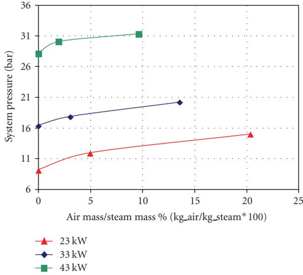
FIGURE 6: Noncondensable gas concentration effect on system pressure [14].
