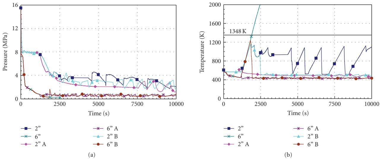
FIGURE 7: LOCA with manual actuation of SI: (a) RCS pressure, (b) core cladding temperature.
