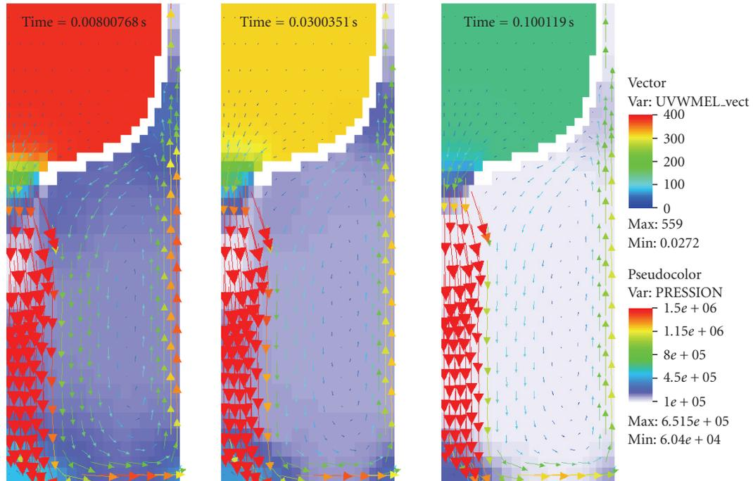
FIGURE 5: Illustration of pure gas flow computed with MC3D at three different times with DISCO P'4 "2D" geometry (background colour according to pressure).
