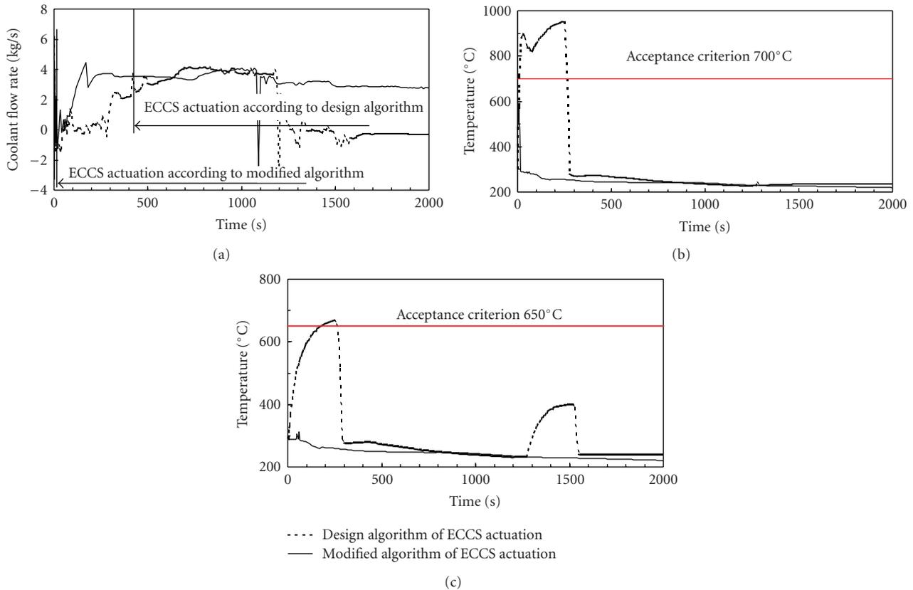
FIGURE 2: Analysis of partial GDH rupture considering modification of ECCS algorithm: (a) coolant flow rate through fuel channels, (b) fuel rod cladding temperature in high-power channel connected to ruptured GDH, and (c) behavior of fuel channel wall temperature.
