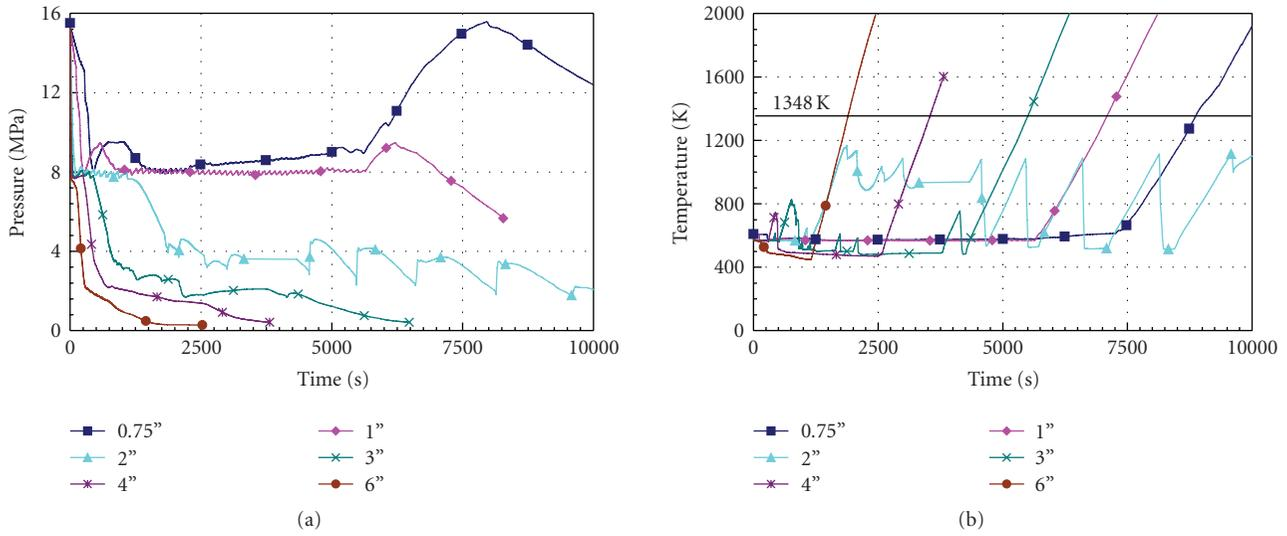
FIGURE 6: LOCA spectrum without SI actuation: (a) RCS pressure, (b) core cladding temperature.
