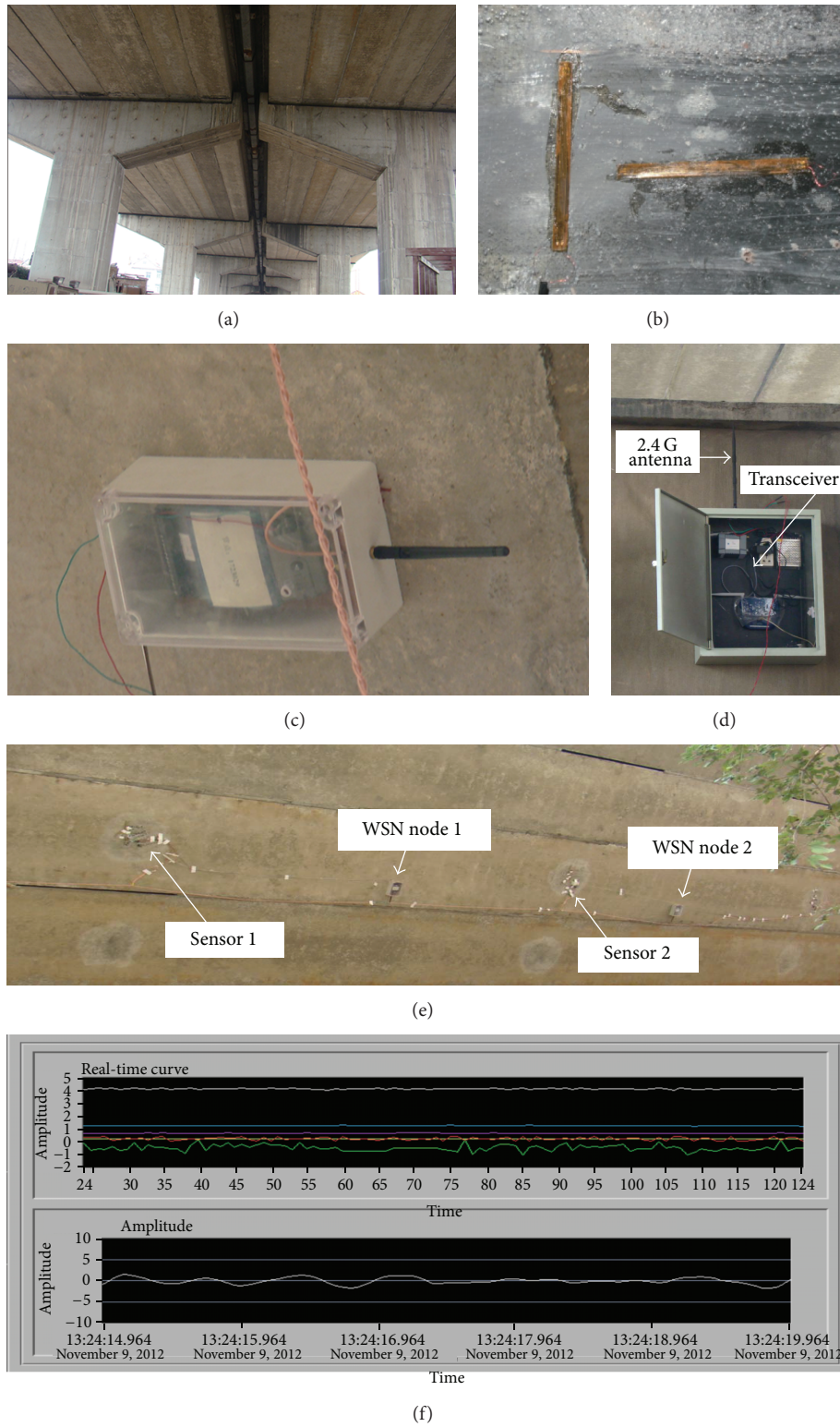
FIGURE 4: (a) The underbridge condition of the Xiaozhang Highway Bridge, (b) strain gauges, (c) WSN nodes, (d) the collection node box, (e) installed network nodes, and (f) the interface of data collection.
