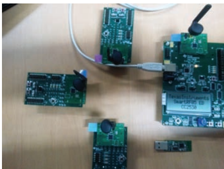
FIGURE 3: 6LoWPAN home nodes based on TI CC2530.
