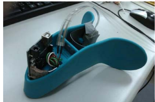
FIGURE 2: The noninvasive wireless sensor PFMT device.
