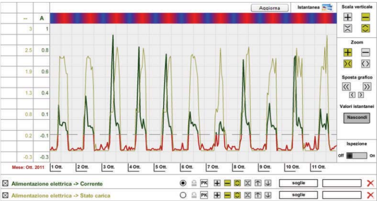
FIGURE 8: Current draw and charge status of SNU 1 from October 1st to October 11th.
