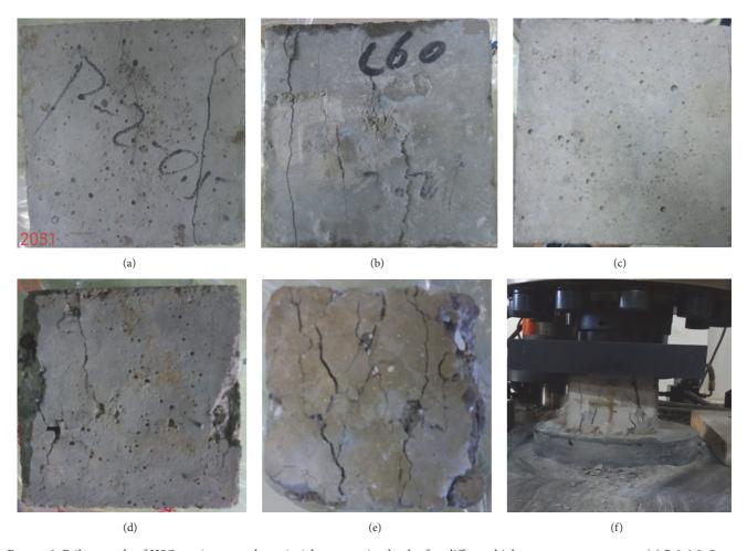
FIGURE 3: Failure mode of HSC specimens under uniaxial compression loads after different high temperature processes: (a) P-2-0.5,  $S_{\max} = 0.80, 0.5N_f$ ; (b) P-2-3,  $S_{\max} = 0.85, 0.5N_f$ ; (c) P-5-0.5,  $S_{\max} = 0.90, 0.25N_f$ ; (d) P-6-3,  $S_{\max} = 0.85, 0.75N_f$ ; (e) P-8-2,  $S_{\max} = 0.90, N_f$ ; (f) critical failure state of fatigue.
