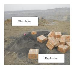
Figure 12: Picture of the field experiment.
