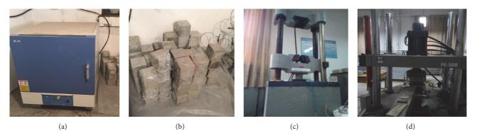
FIGURE 1: Apparatus and specimens: (a) box-type resistance furnace; (b) specimens; (c) electrohydraulic servo pressure machine; (d) electrohydraulic servo fatigue machine.
