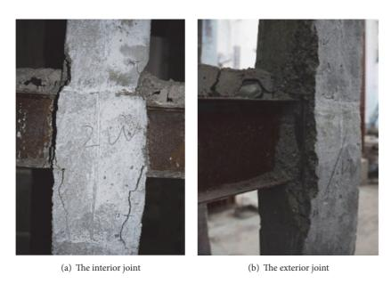
FIGURE 14: Cracks on joints at the second floor.
