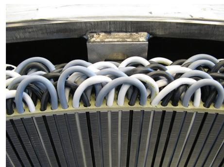
FIGURE 5: The stator winding with white, grey, and black cables used for the three phases.
