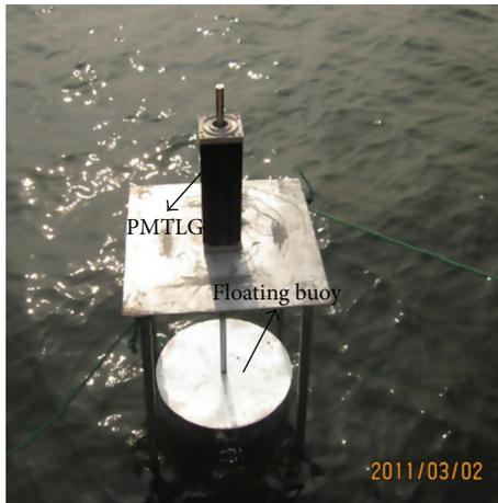
FIGURE 11: A wave energy extraction system was installed in Xuanwu Lake, China (in trial phase).
