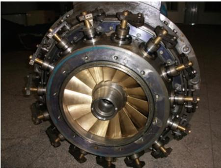
FIGURE 13: Photograph of guide vane.
