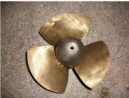
FIGURE 14: Photograph of turbine runner model.
