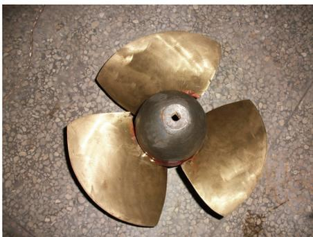
FIGURE 14: Photograph of turbine runner model.
