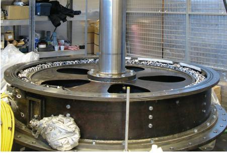
FIGURE 6: The un-magnetized rotor in position resting on the thrust bearing.
