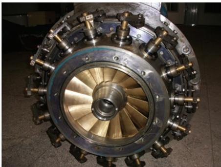
FIGURE 13: Photograph of guide vane.
