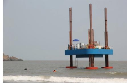
FIGURE 1: *Haiyuan 1* wave power generating jack-up platform.
