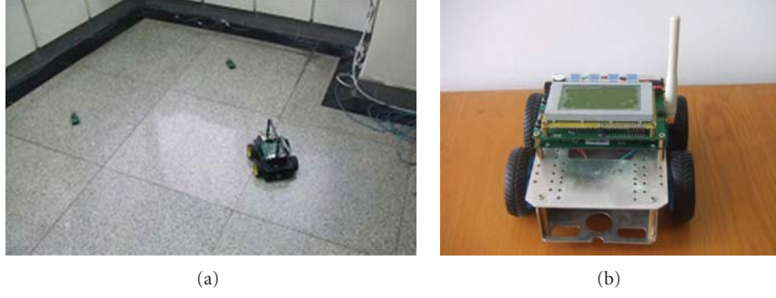
FIGURE 6: (a) Experimental setup to collect data from the static sensor nodes with a mobile sink node moving on a uniform grid. (b) The mobile sink node named DataTruck designed by ourselves.
