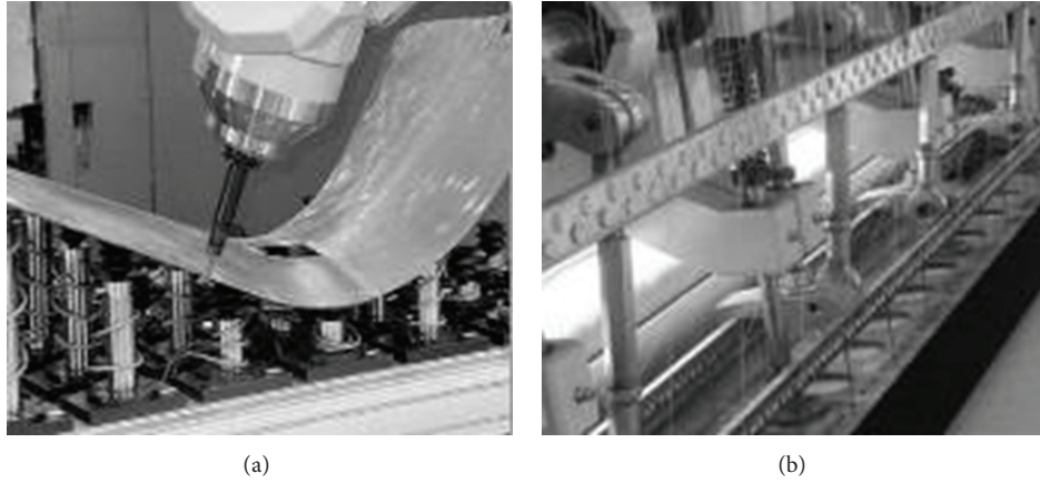
FIGURE 1: FMP example: (a) flexible thin parts processing and (b) quilting processing.
