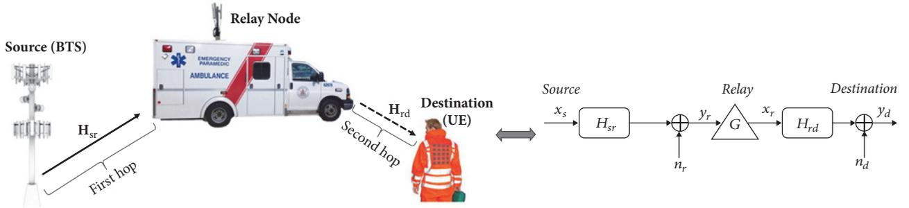
FIGURE 1: System model of a two-hop half-duplex single relay scenario.
