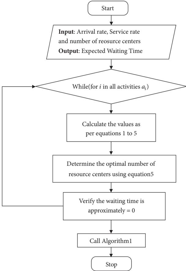
FIGURE 3: Flowchart of the Proposed Resource Scheduling Algorithm 2.
