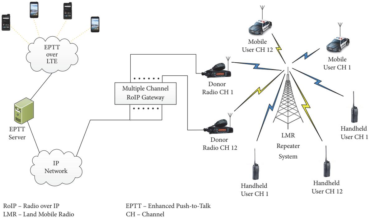
FIGURE 8: PoC to LMR interoperability via RoIP gateway [31].
