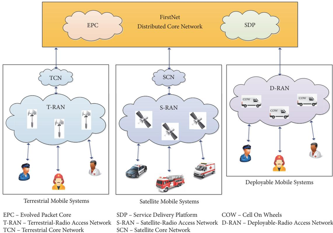
FIGURE 5: FirstNet's architecture for public safety communications.
