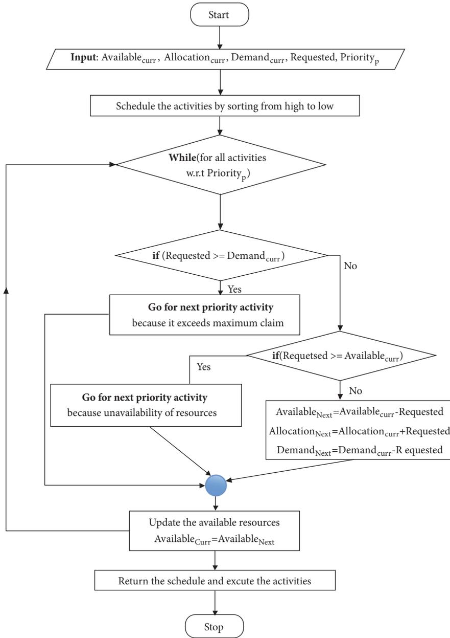
FIGURE 2: Flowchart of the Proposed Resource Scheduling Algorithm 1.
