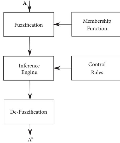
FIGURE 5: Block diagram of Fuzzy Logic Algorithm.
