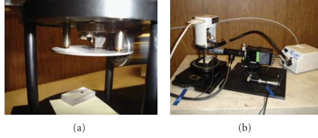
FIGURE 1: Images of the setup. The long-working-distance microscopic lens is pointed at the AFM cantilever.
