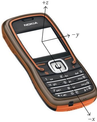
FIGURE 2: Nokia 5500 accelerometer axes.
