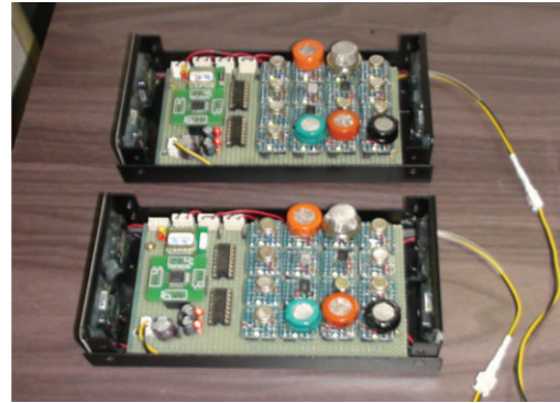
FIGURE 4: Actual image of a stereo sensor array for odor data acquisition.
