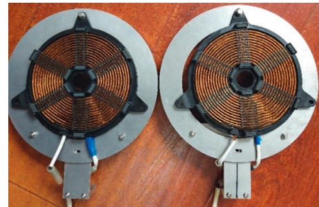
FIGURE 13: Receiving coil and launch coil of the practical MCRETS system.
