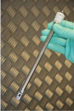
FIGURE 13: Probe sensor for in-vessel monitoring applications.
