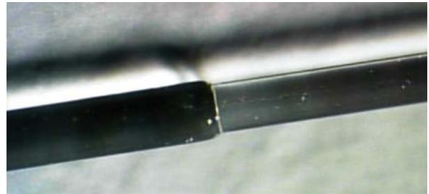
FIGURE 4: One of the two waveguides of the Gemini fiber G2 spliced to a standard telecom fiber through automatic alignment between cladding images.
