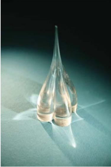
FIGURE 1: Preform of Gemini fiber G4, where four individual standard telecom fiber preforms are mounted together and drawn into a monolithic fiber with four easily accessed ports.
