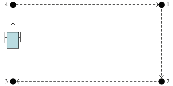
FIGURE 4: Waypoint navigation. A mobile device traverses the sensing region by navigating between position coordinates.
