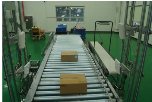
(b) Installed roller conveyor
