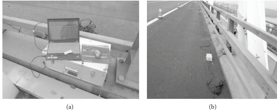
FIGURE 8: Ambient vibration testing of Guanhe Bridge.
