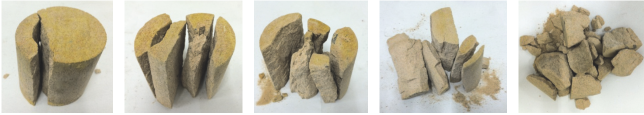
FIGURE 10: Failure forms under different freeze-thaw cycles.
