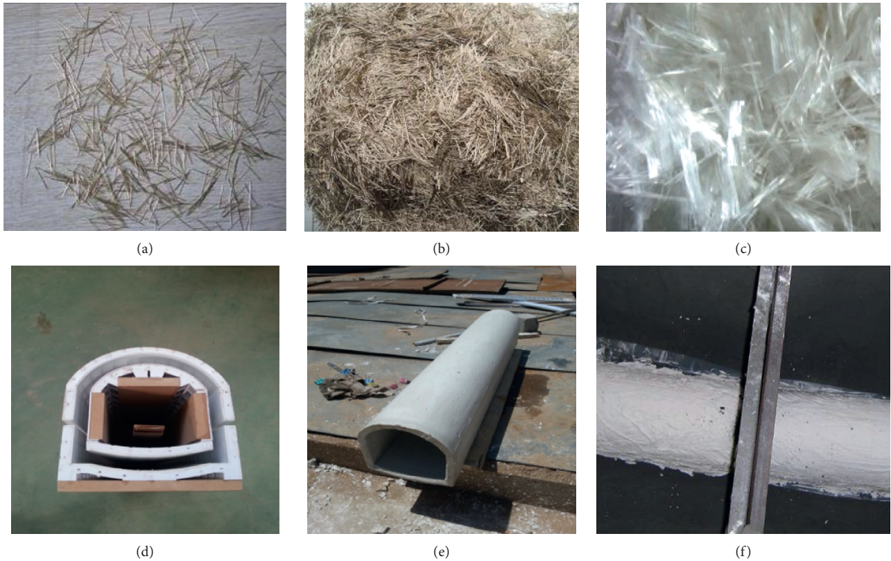
FIGURE 6: Test similar material and model. (a) Steel fiber. (b) Basalt fiber. (c) Polypropylene fiber. (d) Model casting. (e) Model of lining. (f) Waterproof board and primary support.
