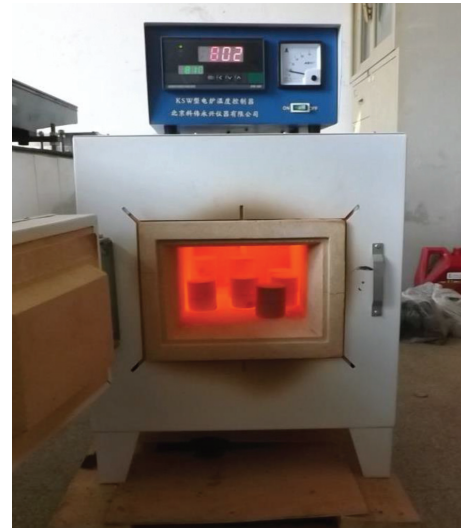
FIGURE 1: Sandstone specimens heated using box-type resistance furnace.
