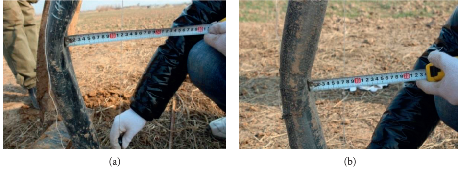
FIGURE 15: Macroscopic deformation of the two pipeline specimens. (a) Standard pipeline. (b) CFRP pipeline.
