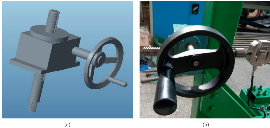
FIGURE 8: Worm screw jack. (a) 3D model of the worm screw jack. (b) Virtual object of the worm screw jack.
