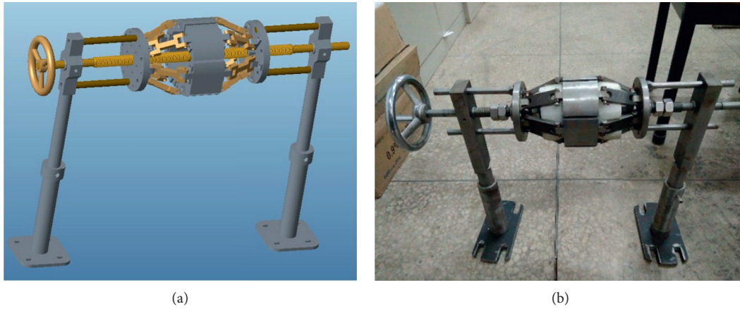
FIGURE 15: Excavation unloading device. (a) 3D model of the excavation unloading device. (b) Virtual object of the excavation unloading device.
