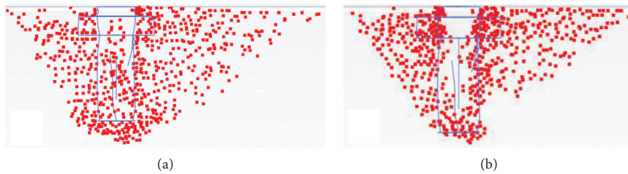
FIGURE 21: Plastic deformation diagram of low-skirted suction caisson under inclined load: (a) \beta = 0^\circ and L = 0 ; (b) \beta = 45^\circ and L = 0 .
