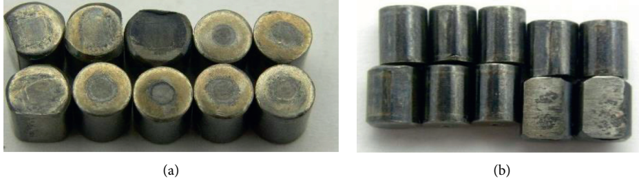
FIGURE 1: Examples of high-speed cylindrical roller bearing failures.
