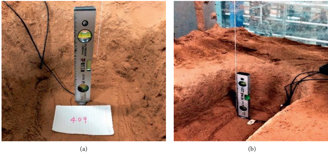
FIGURE 4: Burial diagram of Earth pressure box.
