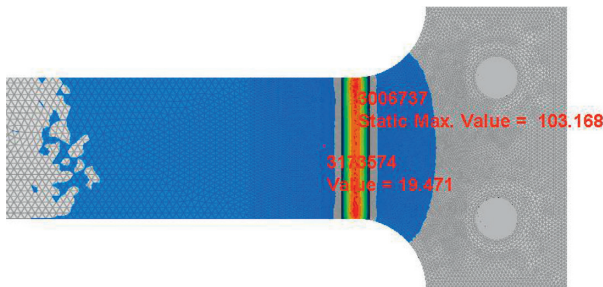
FIGURE 11: Calculation of the stress concentration factor (unit: MPa).
