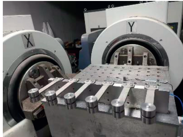
FIGURE 15: Original fatigue life test countertop arrangement.
