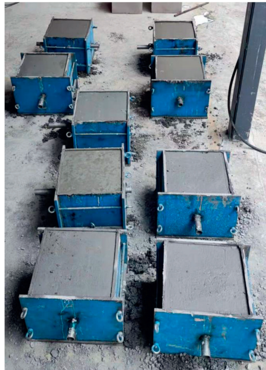
FIGURE 4: Poured concrete blocks.
