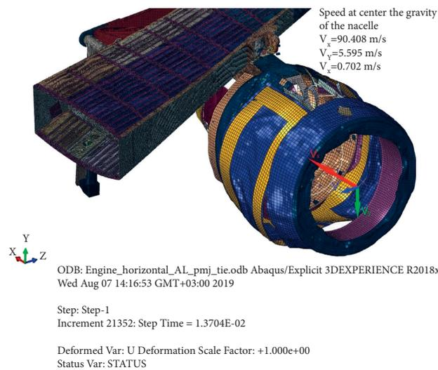
FIGURE 28: Deformation and velocity of center of gravity after emergency disconnection—course of impact.
