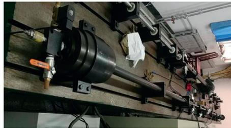
FIGURE 7: Hopkinson bar impact test system.
