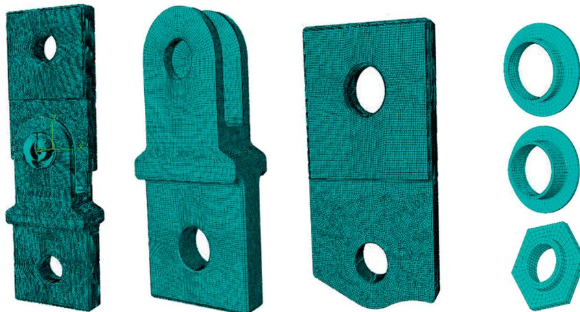
FIGURE 15: Model of emergency fuse pin and attachments.
