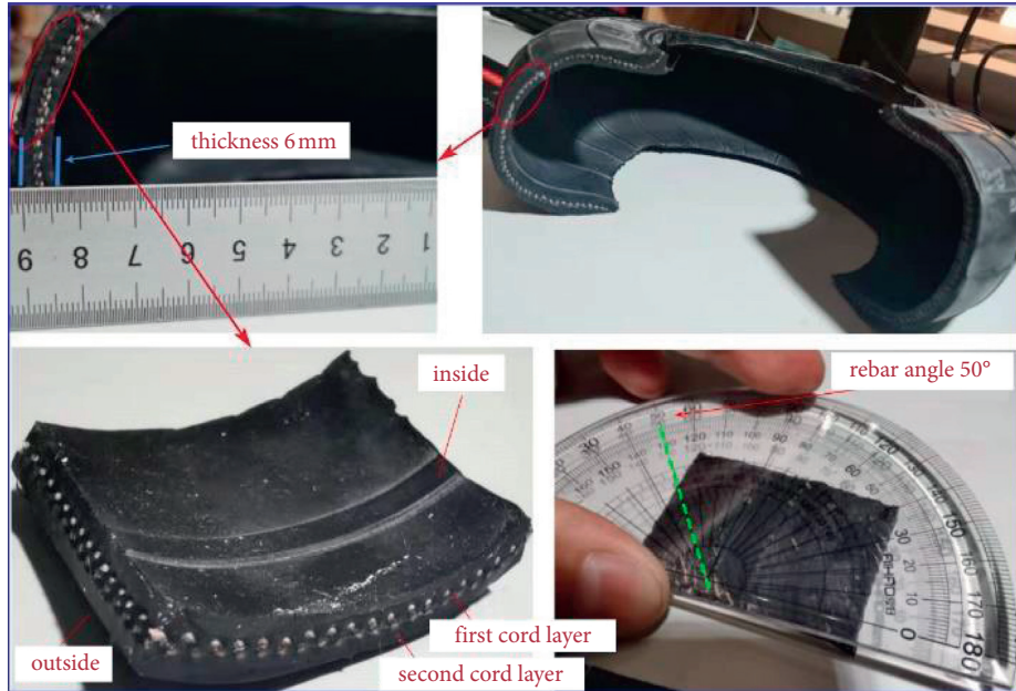
FIGURE 6: Cord distribution of the airbag rubber matrix.
