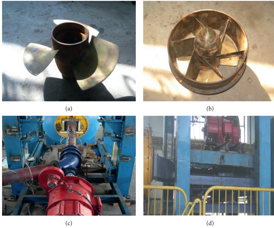
FIGURE 2: Pictures of experiment: (a) impeller; (b) guide vane; (c) physical diagram of test equipment of the axial-flow pump; (d) physical diagram of test equipment of the axial-flow pump device.
