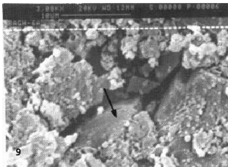
FIGURE 9. SEM photo of Struvite mineral (orthorhombic system), which shows (1) flaky prismatic shape with sharp edges, (2) radial texture grown on or between the flaky prismatic forms, (3) honeycomb-like surface of the mineral Hydroxy apatite.
