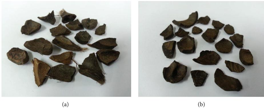
FIGURE 6: Crushed *dura* (a) and *tenera* (b) OPS coarse aggregates.
